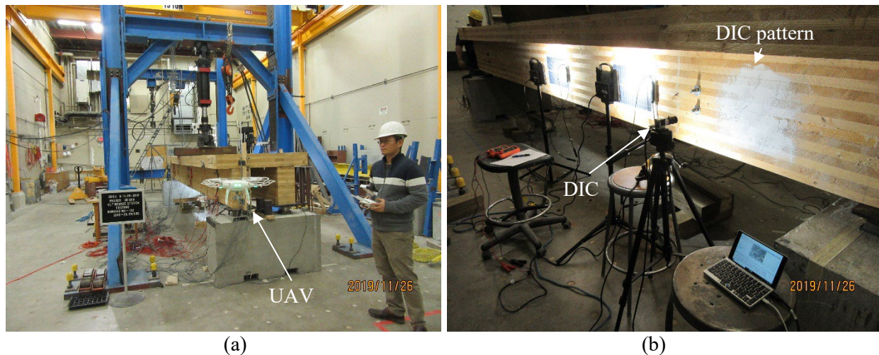
Figure 2.105 Non-contact sensor operation: (a) UAV and (c) DIC system
