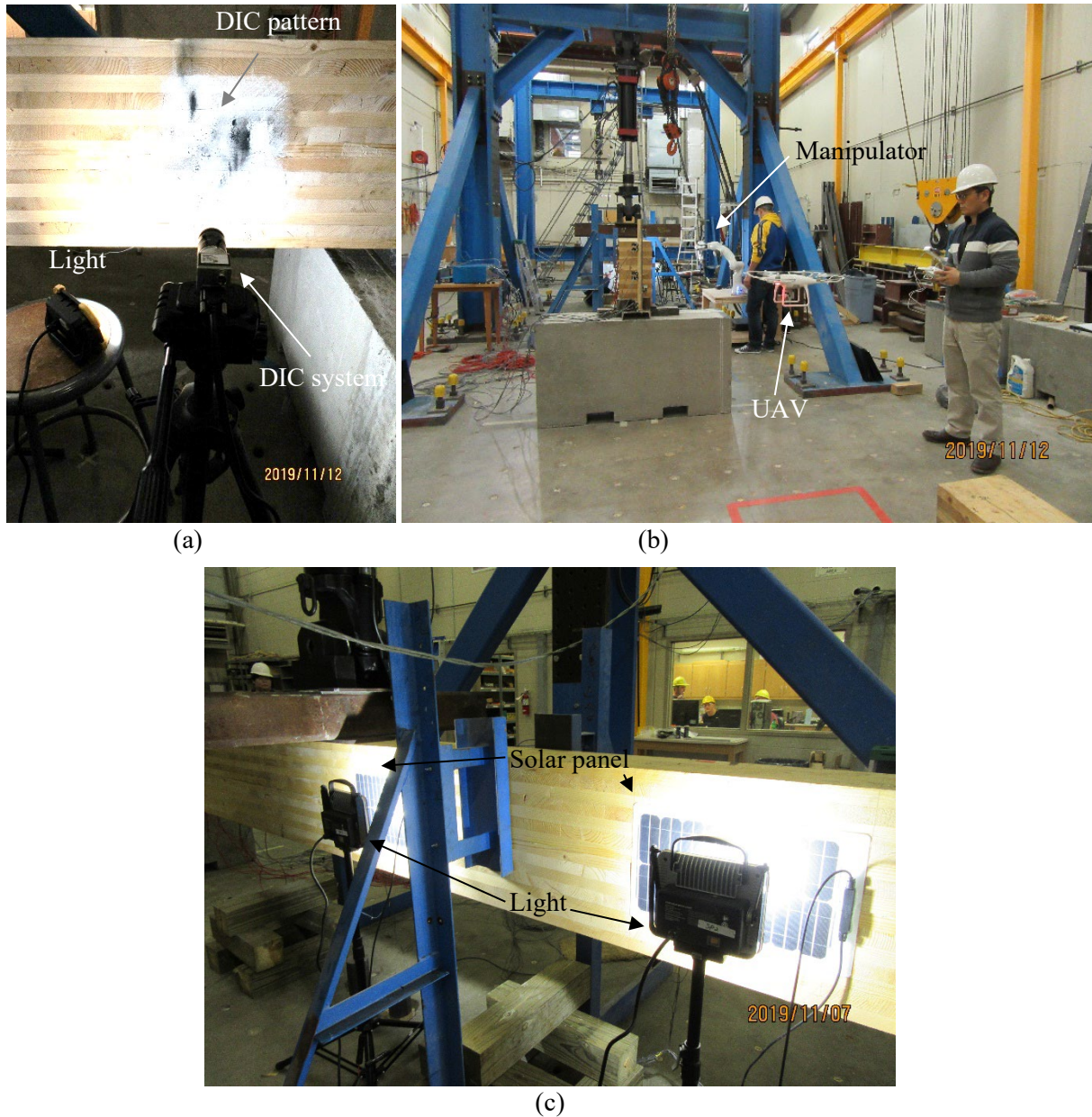
Figure 2.37 Non-contact sensor: (a) DIC system; (b) UAV and manipulator; and (c) solar panel
