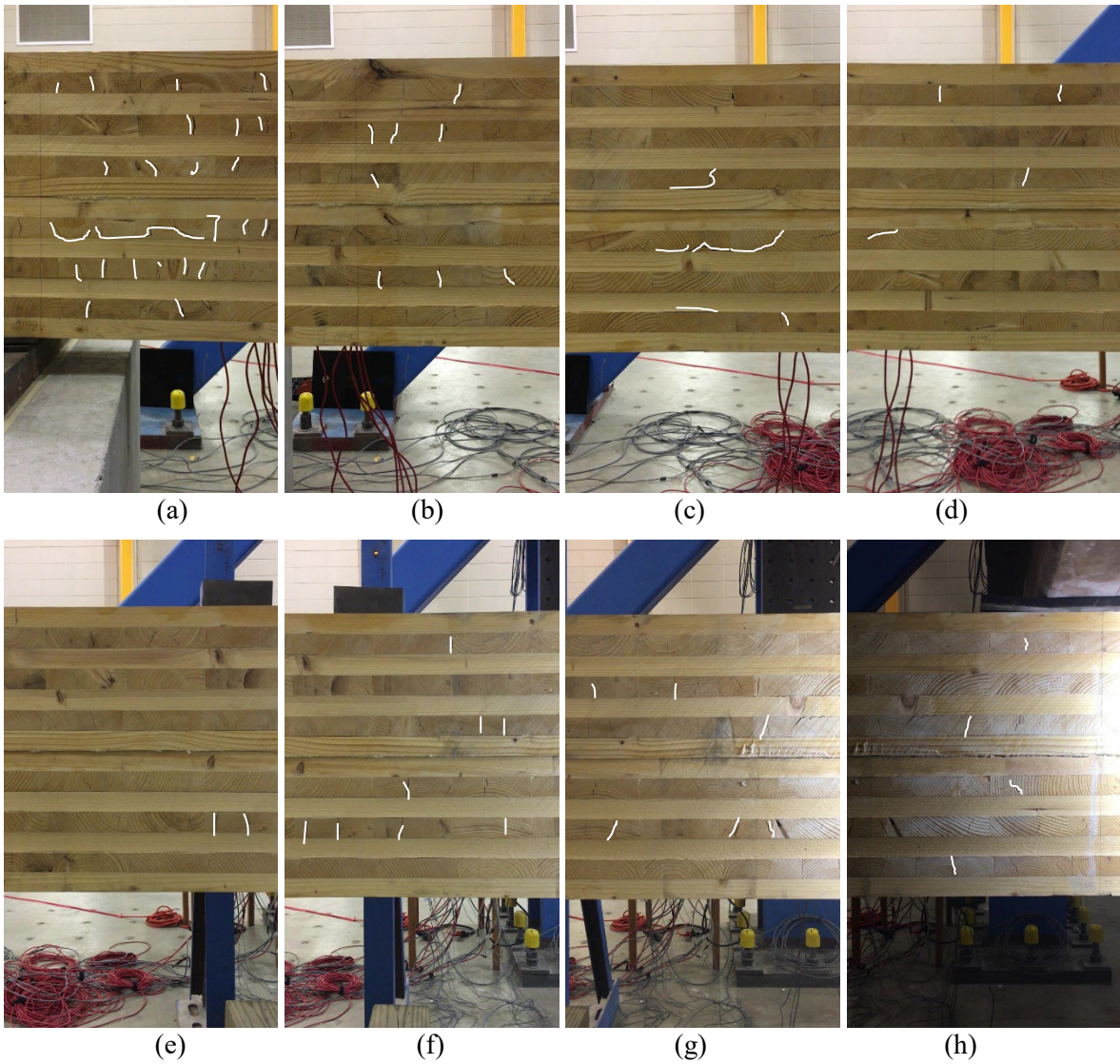
Figure 2.81 Southeast sections of CLT girder before the testing captured by manipulator: (a) section 1; (b) section 2; (c) section 3; (d) section 4; (e) section 5; (f) section 6; (g) section 7; and (h) section 8
