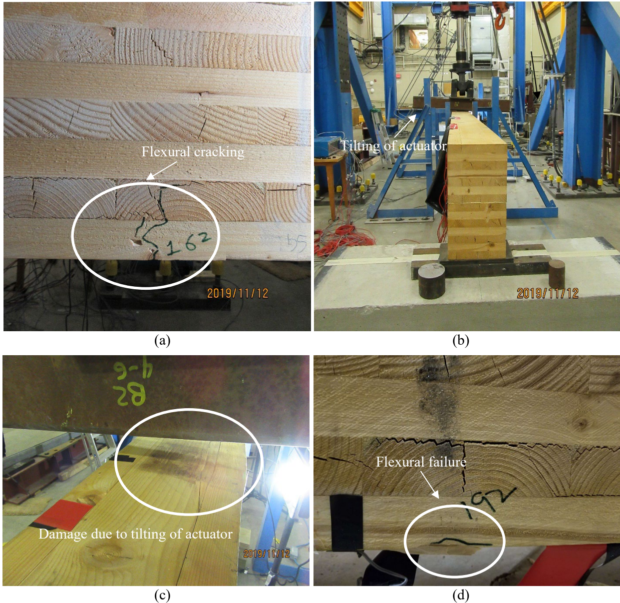
Figure 2.67 Representative damage images: (a) flexural cracking on the east side of the girder at mid-span; (b) tilting of actuator; (c) damage due to tilting of actuator; (d) flexural failure on the west side of the girder at mid-span
