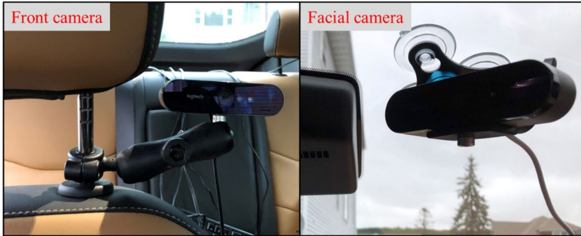
Figure 29. Front Camera and Facial Camera Placement
