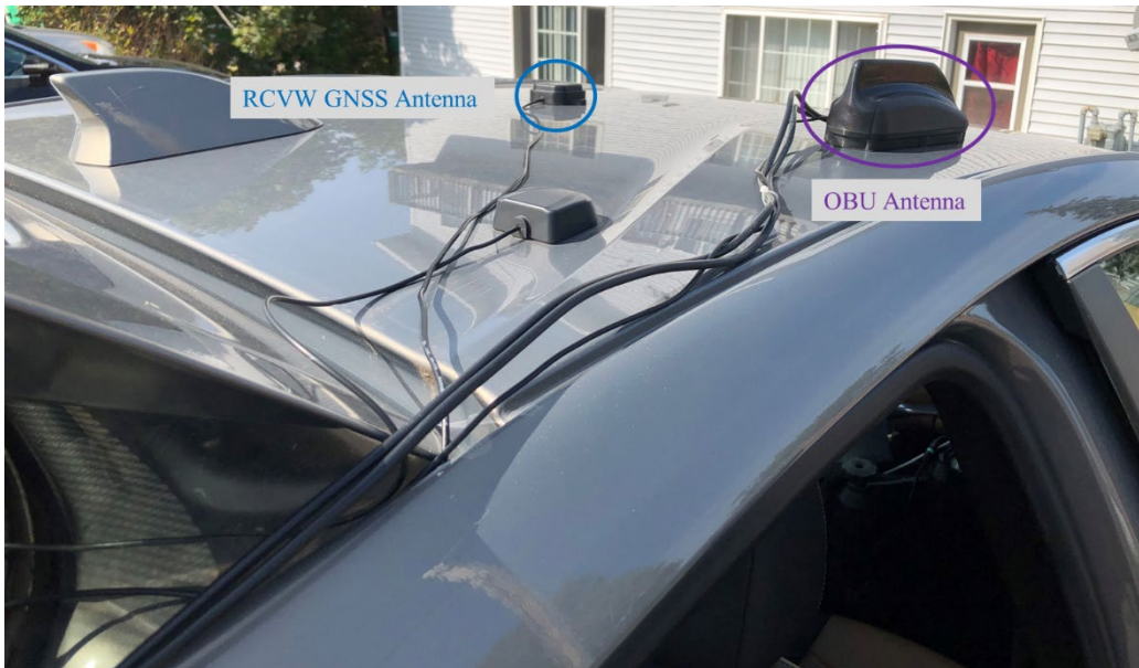
Figure 28. VBS Antennas Placement
