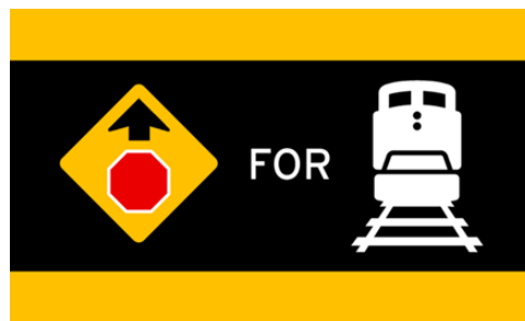
Figure 15. Active Crossing Ahead Alert
