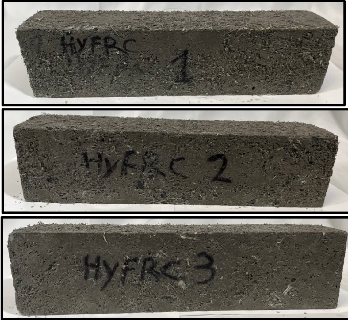
Figure 40. HyFRC samples after 300 cycles
