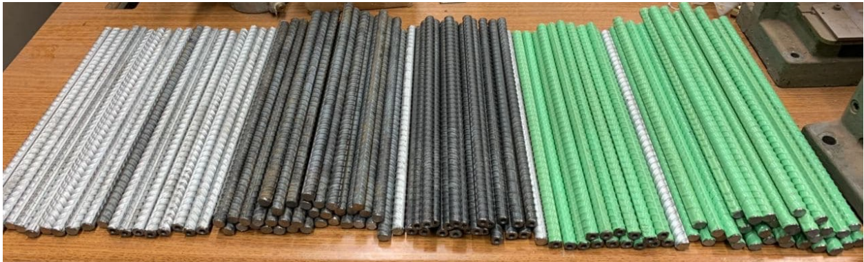
Figure 4. Galvanized, black, ChromX and epoxy-coated bars
