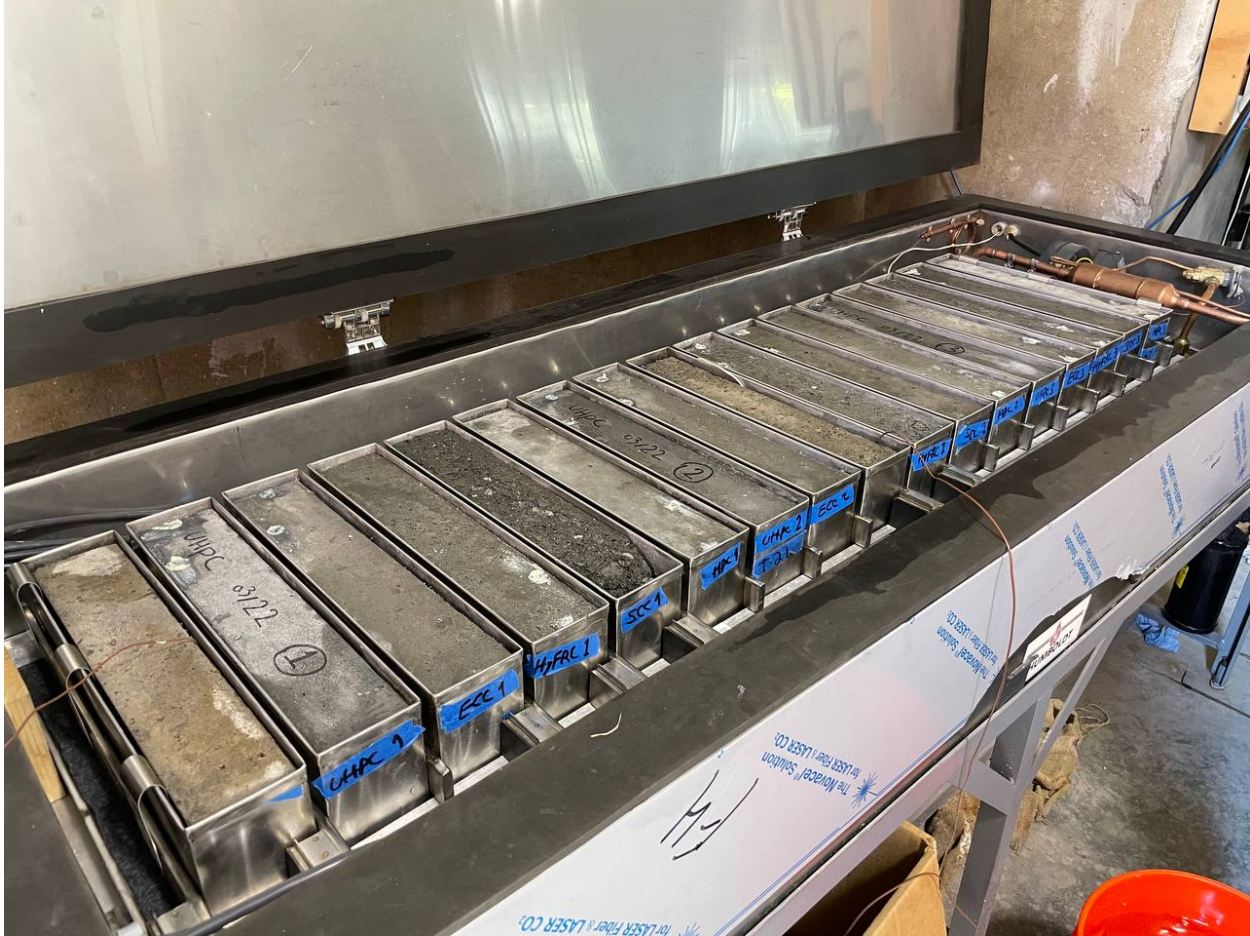
Figure 31. Specimens in the freeze-thaw machine
