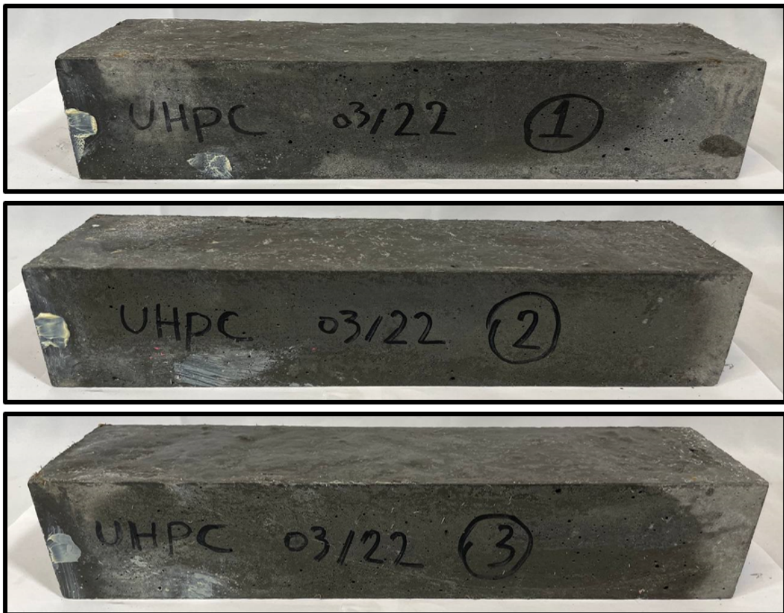
Figure 42. UHPC specimens after 300 cycles
