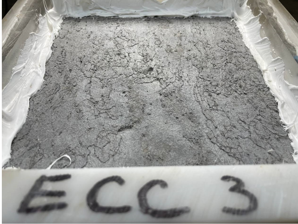
Figure 50. Scaling damage in ECC sample three
