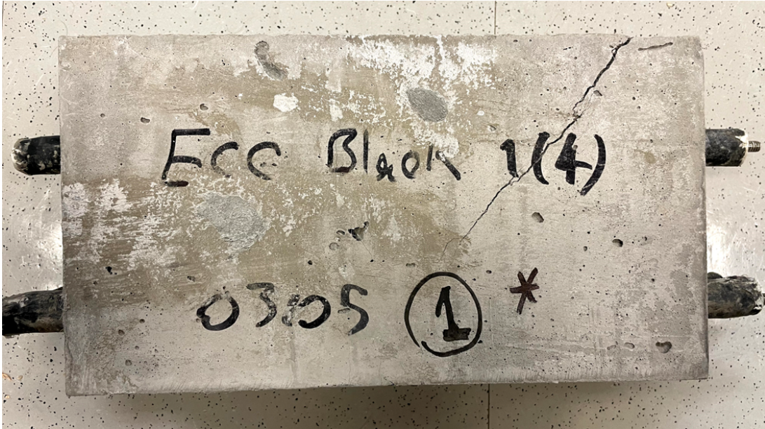
Figure 12. Large shear crack in the failed ECC specimen
