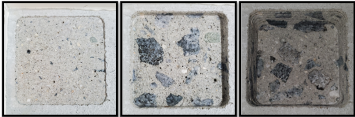
Figure 9. Ground specimens in different depths
