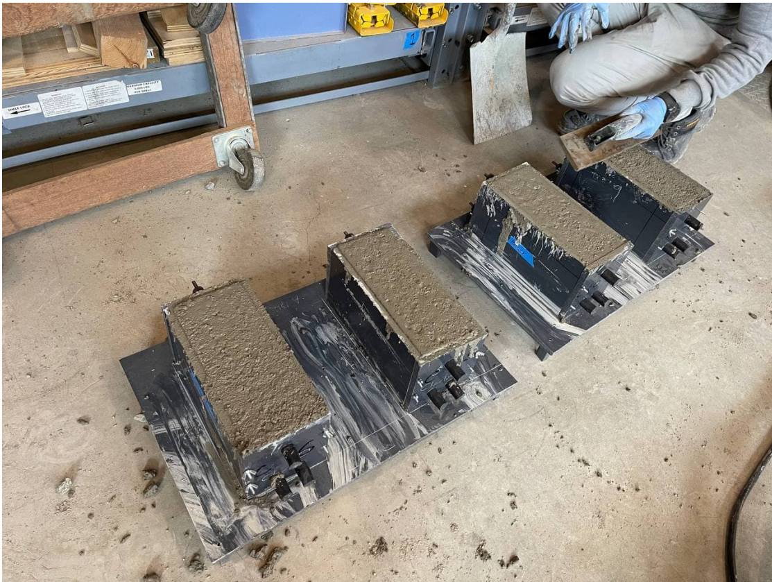
Figure 8. G109 Beam after Casting
