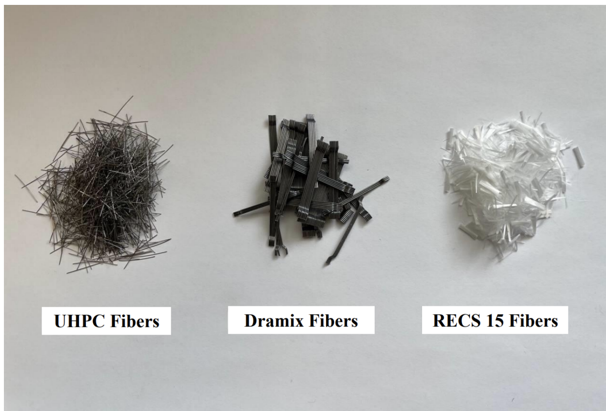
Figure 3. Steel and PVA fibers
