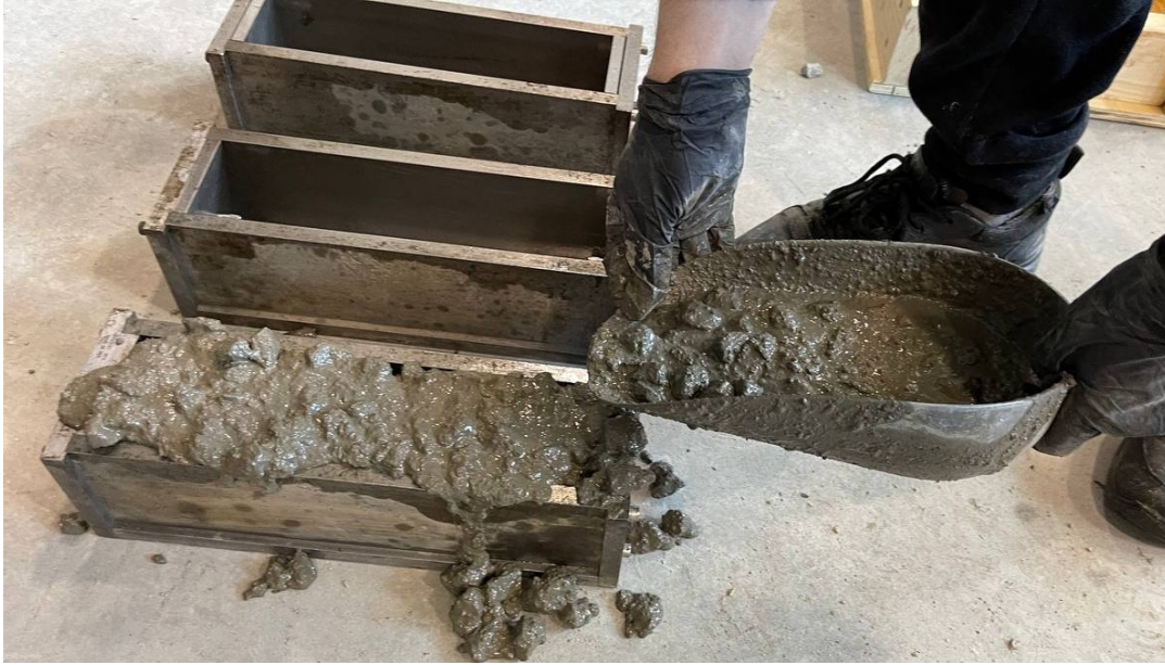
Figure 52. Casting SCC P in drying shrinkage molds
