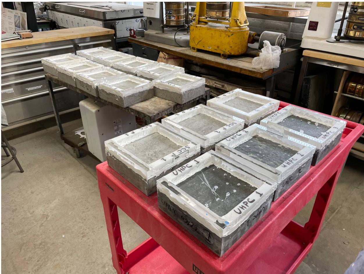
Figure 32. Salt scaling specimens ready to be ponded
