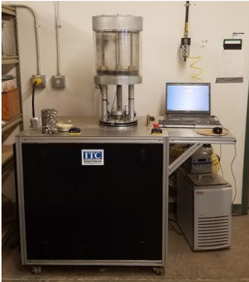
Figure 5.1 SPT test device. Chiller unit is the grey unit on the bottom right of the image. The chiller unit operates correctly but is incapable of serving as an effective heat removal pump for the test device as the test device overheats.
