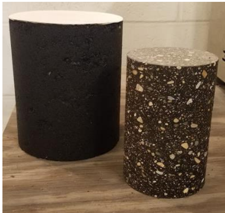
Figure 5.2 Gyratory Specimen and final cored specimen comparison.
