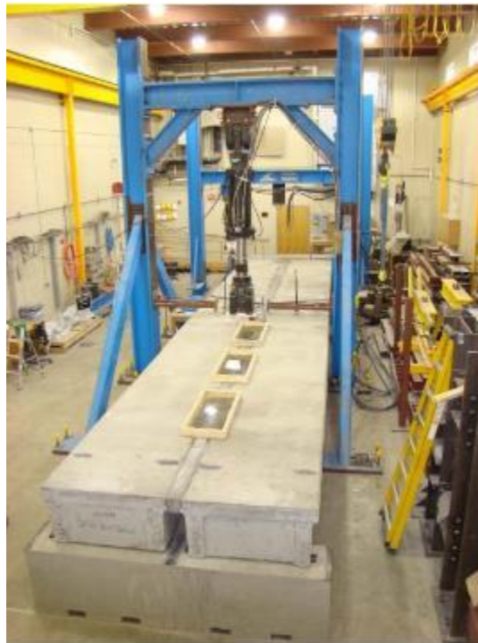
Figure 2-3. Full-Scale Conventional Double-Tee Girder Test Specimen (after Konrad, 2014)
