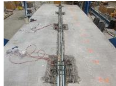
f. Pocket Reinforcement
