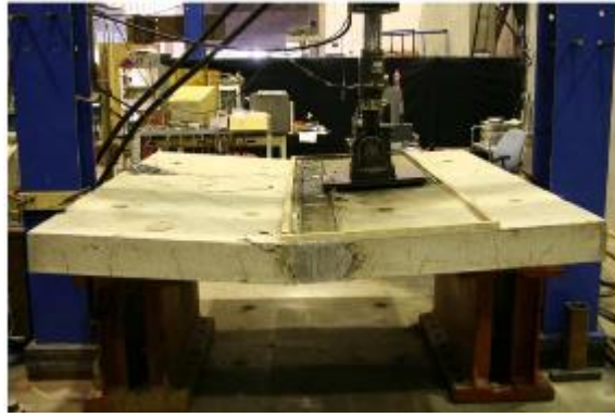
Figure 5-5. Failure of Longitudinal Deck Panel-to-Panel Joint with Straight Bars under Fatigue Loading (after Graybeal, 2010)
