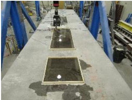
Figure 7-17. Water Dams on Rehabilitated Joint of Double-Tee Bridge Test Specimen
