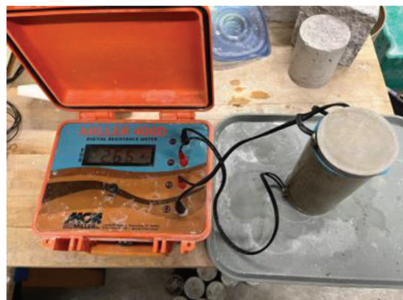
Figure 6.1 The setup of resistivity measurement.
