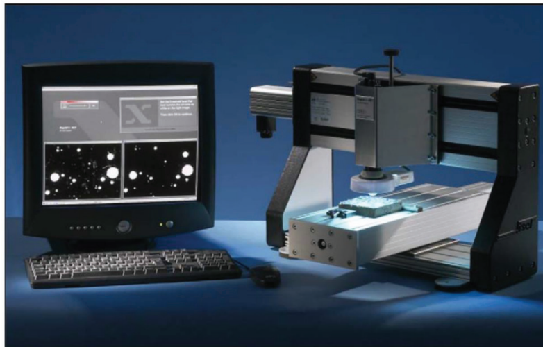
Figure 8.1 The RapidAir system for automatic analysis of the air void system in hardened concrete (Jakobsen et al., 2006).
