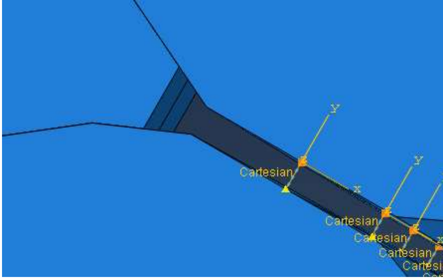
Figure 11: The connectors placed between the interaction surfaces of the wires and their local coordinates. The x, y, z axis of the local coordinates is referred as U1, U2, and U3 directions in this report.
