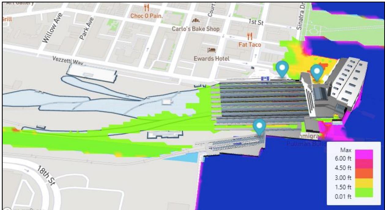
Figure 6 The 3-D Map module showing a top-down view of 1) the base map, 2) the Hoboken Terminal Facility, 3) a frame of animated flood scenario, and 4) the asset extrusions.
