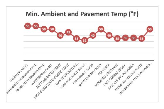
Figure 43 Minimum Ambient and Pavement Temperature (°F) Requirements for Various Marking Materials
