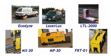
Figure 70 Examples of Portable Retro-reflectometers in TxDOT
