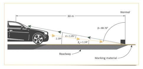
Figure 50 Geometry of Retroreflection (Transports Quebec, 2019)
