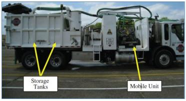
Figure 73 High-Pressure Water Blasting Removal Truck
