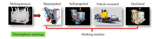
Figure 64 Equipment Required for Thermoplastic Marking (Xu et al., 2021)
