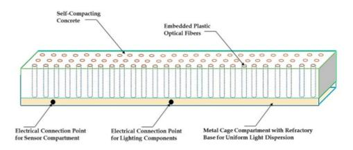
Figure 35 Smart Lane Separator with Detailed Function Description (B)
