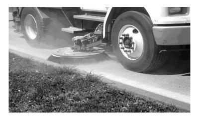
Figure 60 A Typical Broom Truck for Surface Preparations in Texas, New York, and Several Other States.
