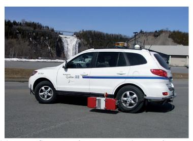
Figure 52 Mobile Retroreflectometer (Transports Quebec, 2019)
