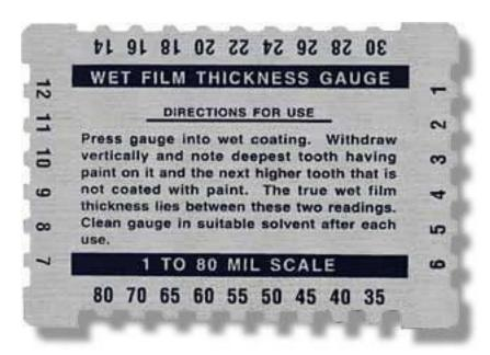
Figure 46 Wet Film Thickness Gauge
