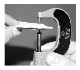
Figure 44 Needlepoint Micrometer Measuring a Thermoplastic Sample (TxDOT, 2004)
