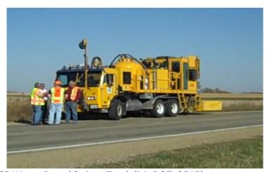
Figure 65 Water Based Striper Truck (MnDOT, 2015)
