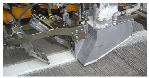
Figure 29 Rib Line Application Method
