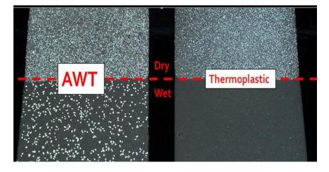
Figure 33 All-Weather Thermoplastic Versus Normal Thermoplastic Both in Dry and Wet Conditions (Source: Yeng Hsingh Co., Ltd, 2020)
