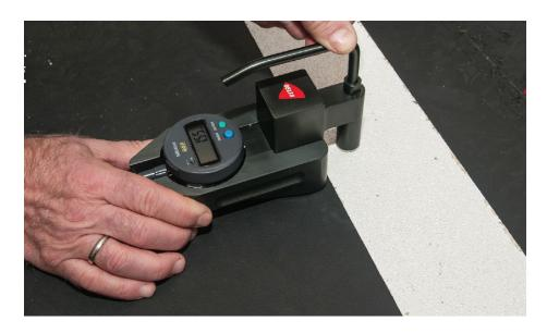
Figure 45 Marking Thickness Gauge (Delta and Forcetechnology, 2014)
