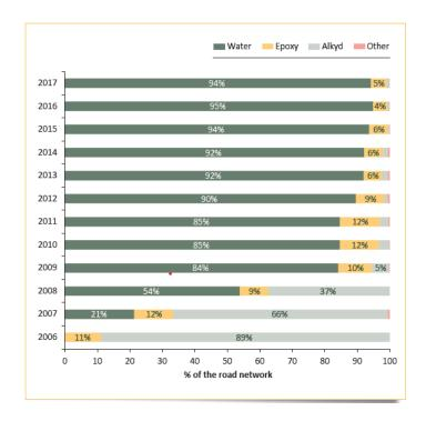
Figure 20 Evolution of the Marking Products Used at the Quebec Ministry of Transportation (Transports Quebec, 2019)
