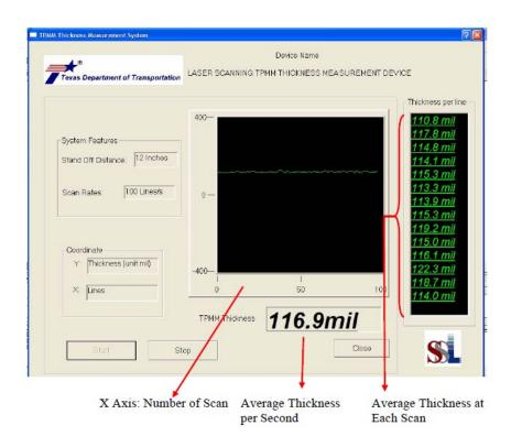
Figure 48 Thickness Information Display (Liu et al., 2006)
