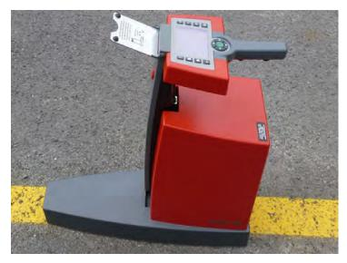
Figure 51 Hand-held Portable Retroreflectometer (Transports Quebec, 2019)
