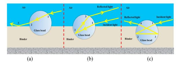
Figure 49 Retroreflection of Glass Beads in Pavement Markings: (a) Too shallow; (b) Suitable; (c) Too deep (Grosges, 2008)
