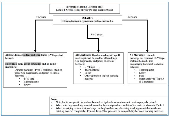
Figure 5 Pavement Marking Selection Process by VDOT
