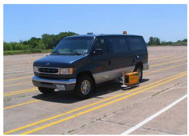
Figure 71 A Typical Pavement Marking Retro-reflectivity Measurement Device by FHWA 5.2.3.2 Equipment Ability to Measure Color of Pavement Markings in Texas and Other States
