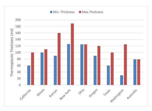
Figure 19 Thermoplastic Application Thickness Across Several U.S. States and Australia
