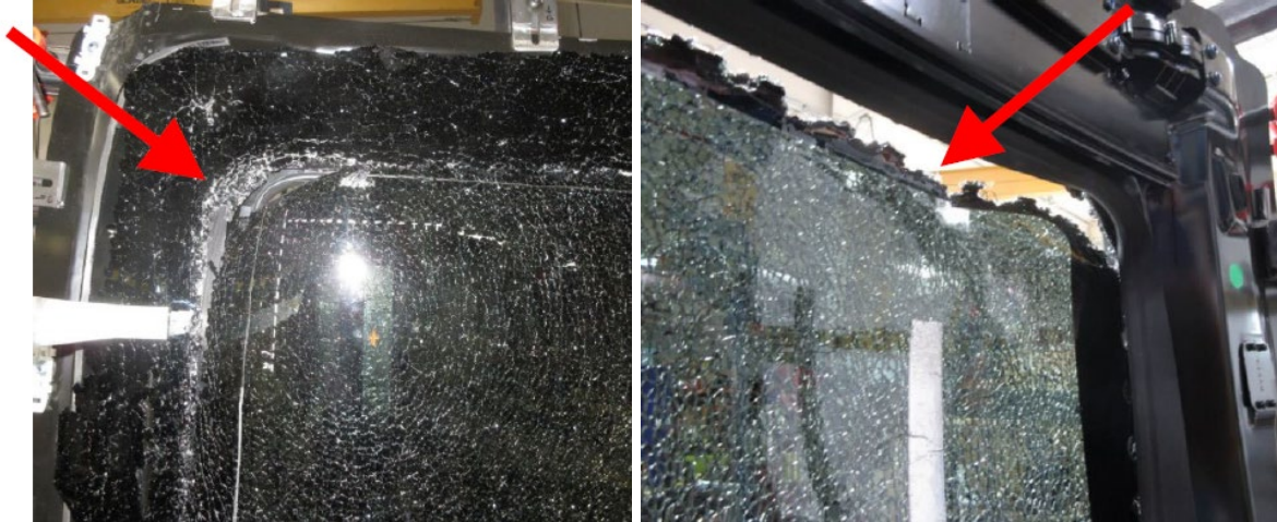
Figure 21. Lincoln MKZ Production Film Layer Rip
