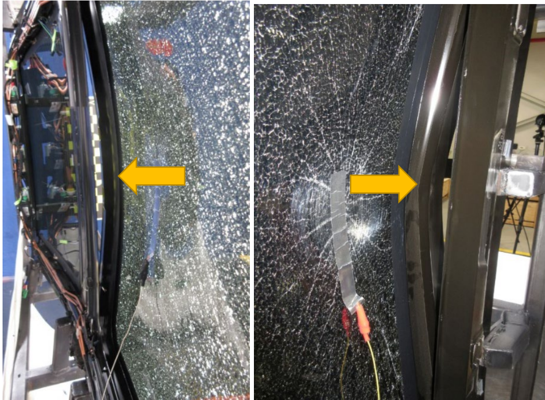
Figure 31. Bending of Metal Frame Holding Glass (Yellow Arrows)
