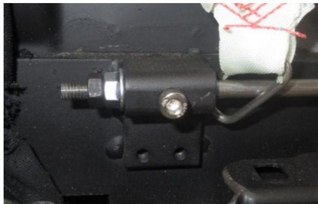
Figure 6. Bolt Attachment of Bottom Guide Rod to Module
