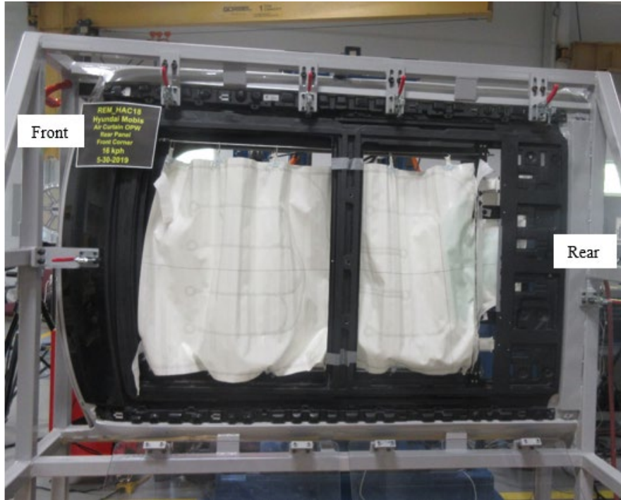
Figure 17. Curtain Manually Opened Across Both Openings Prior to Test
