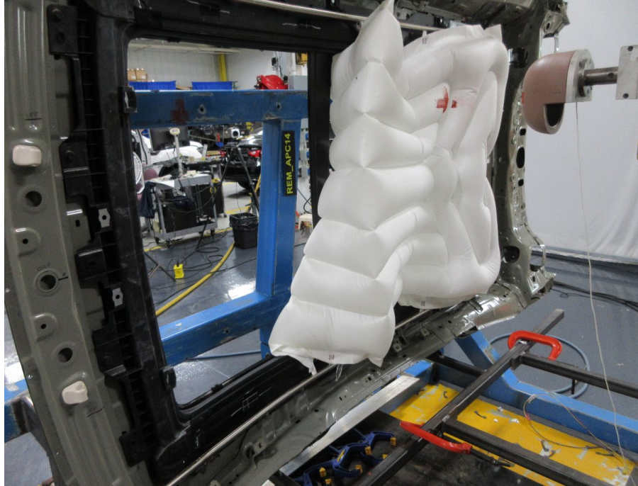
Figure 33. Example of Bag Caught on Middle Support Member
