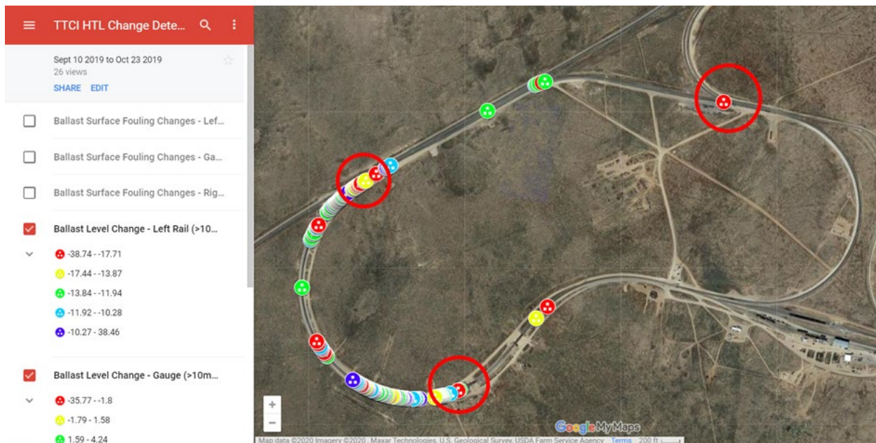
Figure 21. Ballast Height Changes per Meter of Travel (Sept. 10 vs. Oct. 23)
