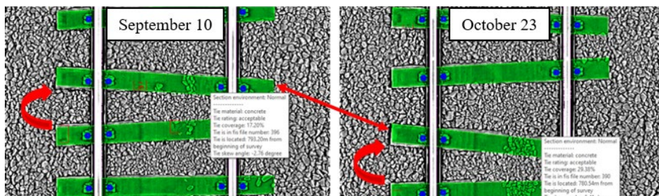
Figure 34. Example of Crosstie Skew Angle Increase
