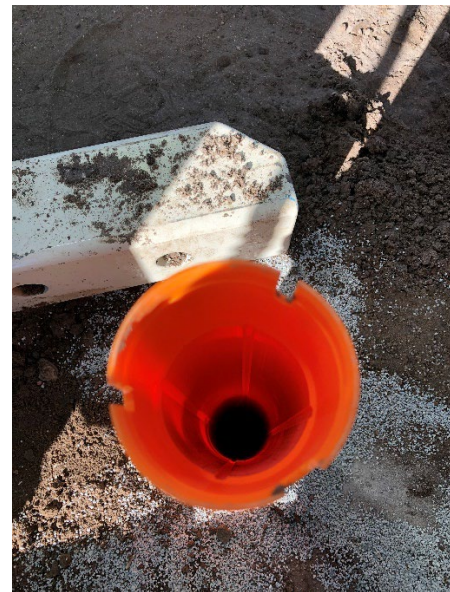
Figure 3.22: Orthogonal Grooves in each Casing (left figure retrieved from Inclinometer Manual)
