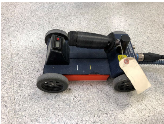
(a) GPR device on concrete
