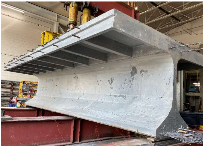
Figure 5.21: Vertical shear test setup and instrumentation
