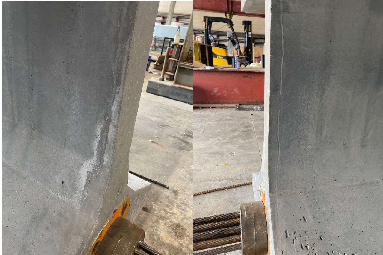
Figure 5.40: Specimen ends after post-tensioning showing no cracking
