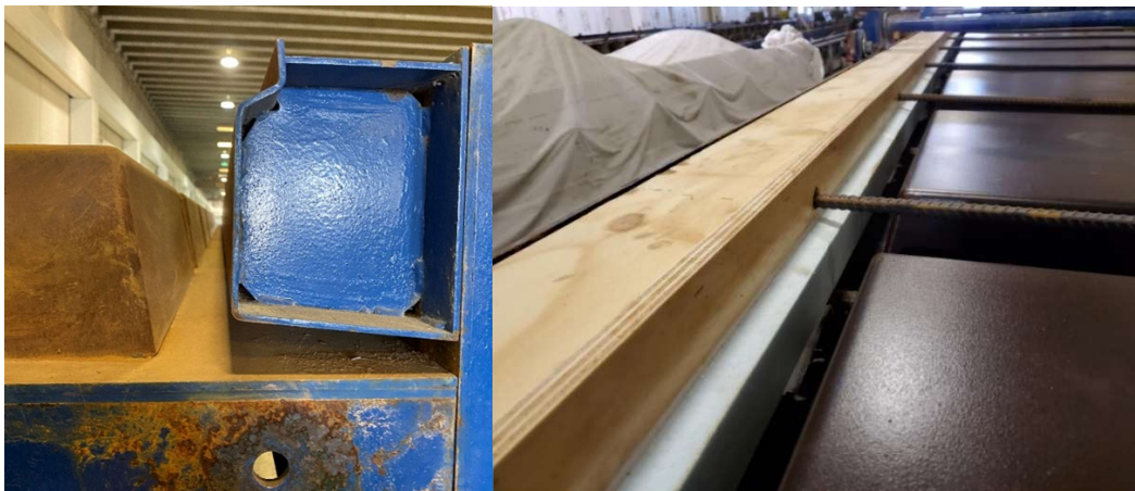
Figure 4.3: Forms and reinforcement of UHPC pretensioned specimen
