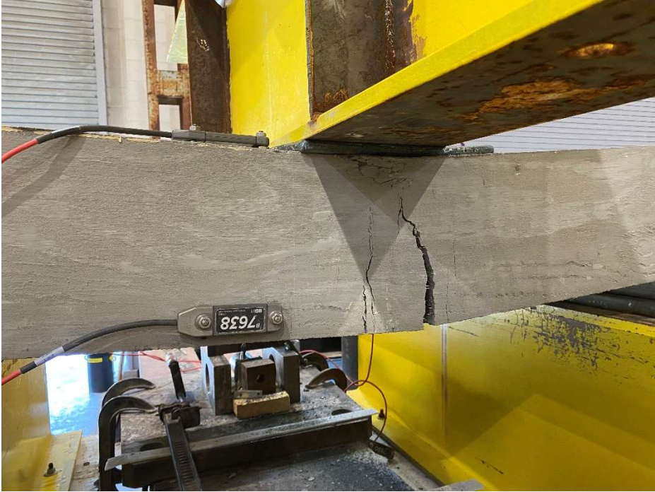
Figure 5.9: Flexure failure mode of the UHPC ribbed slab in negative moment
