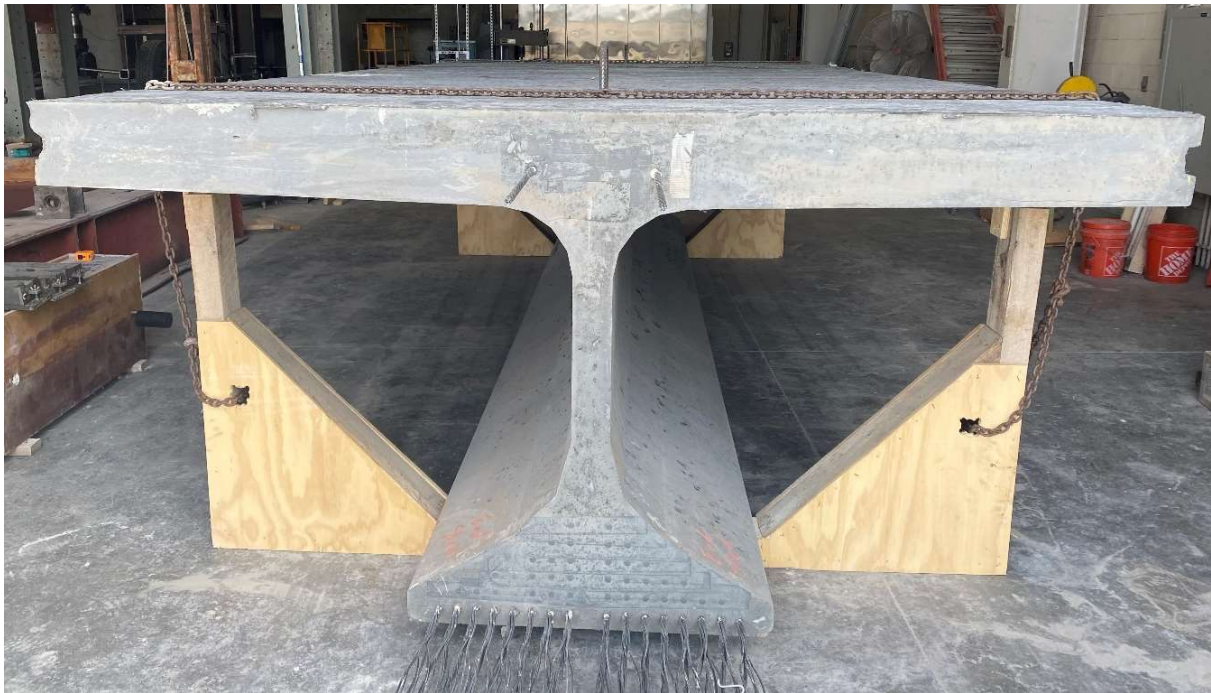
Figure 4.9: Specimen bracing during transportation (top) and storage at the structural lab (bottom)
