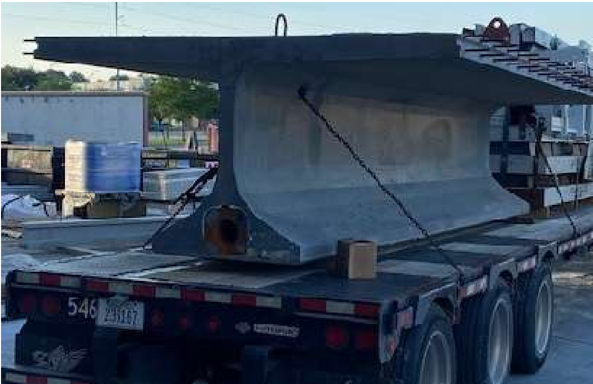
Figure 4.31: UHPC DIB specimen bracing during transportation
