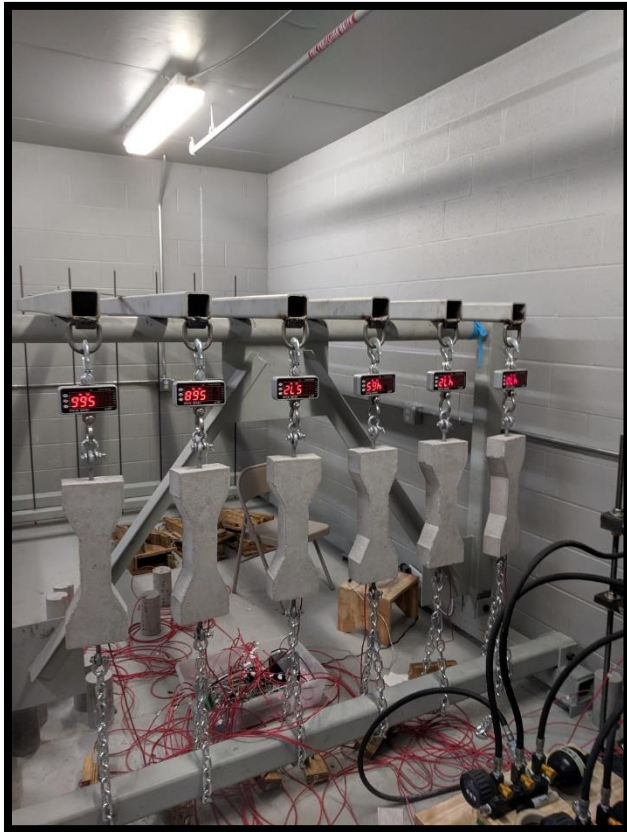
Figure 5.3: Dogbone Specimens Loaded in the Tensile Creep Frame
