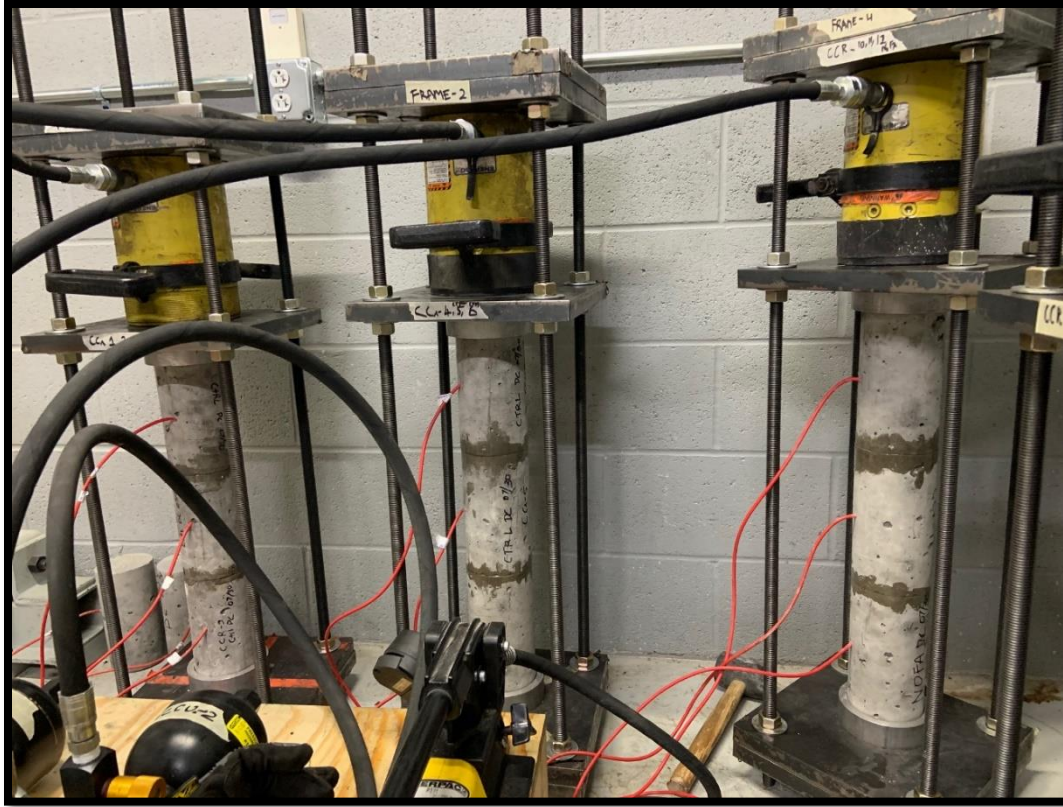
Figure 5.4 Compression Creep Frames Loaded with Concrete Cylinder Specimens
