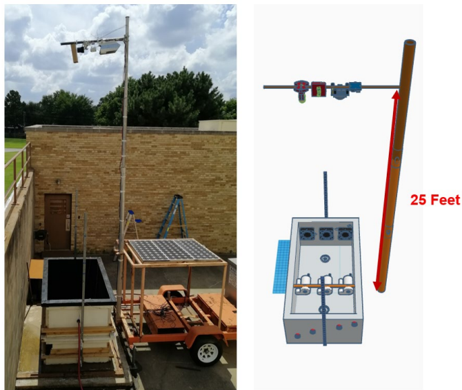
Figure 8. Water-side setup using adjustable pole.
