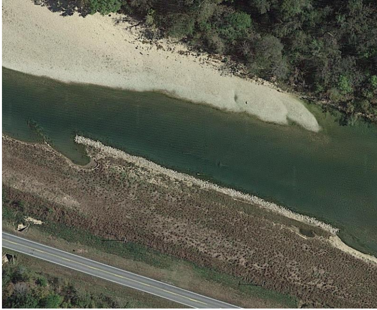
Figure 10: Aerial photo of rock vane in the Illinois River near Tahlequah, OK (GoogleEarth 2020).
