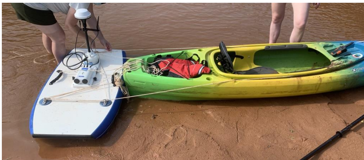
Figure 14: ADCP attached to back of kayak for cross sections in non-wadable rivers.
