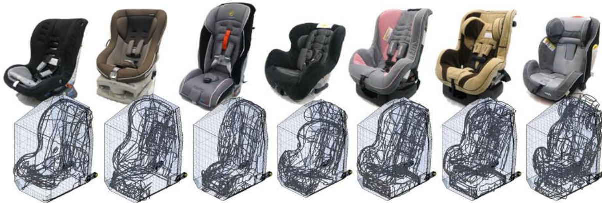
Figure 13. Examples of CRS scans in one of the ISO envelopes (Hu et al., 2015)
