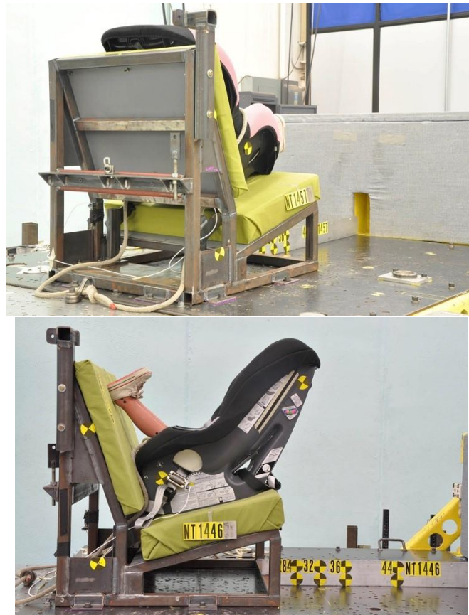
Figure B-1. 2014 version of the updated 213 bench used for the test series
