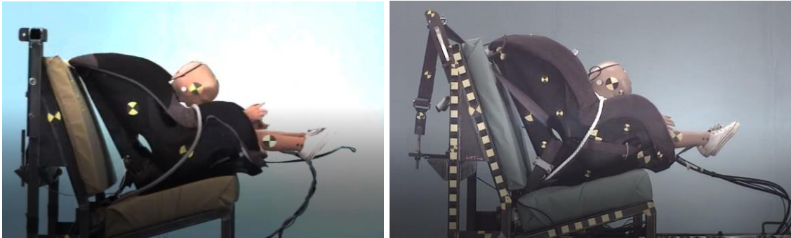
Figure 21. Comparison of peak head excursion from tests NT1419 (left) and NT2102 (right)
