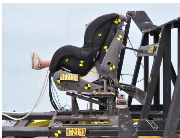
Figure 18. Illustration of vehicle seat mounted rear-facing on FMVSS No. 213 bench
