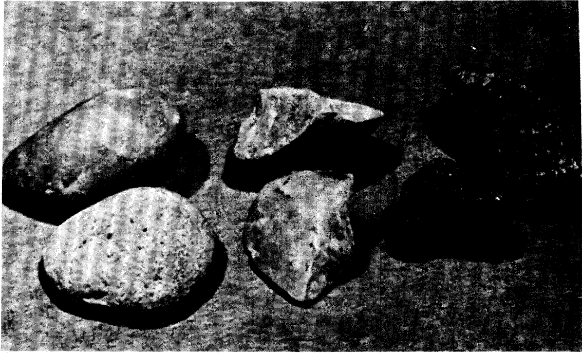
FIGURE 2.31—Aggregate of Various Shape and Surface Textures.
