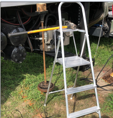
The hammer impact method to sense pile depth uses a simple sledgehammer.
