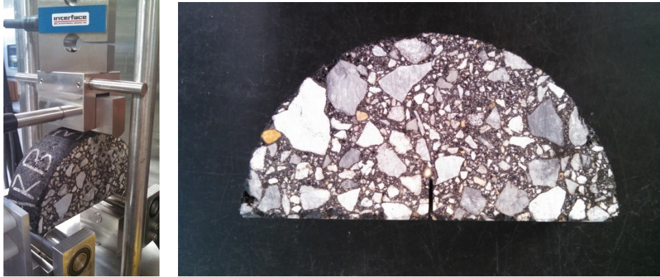
Figure 6. I-FIT Test Setup and Specimen
