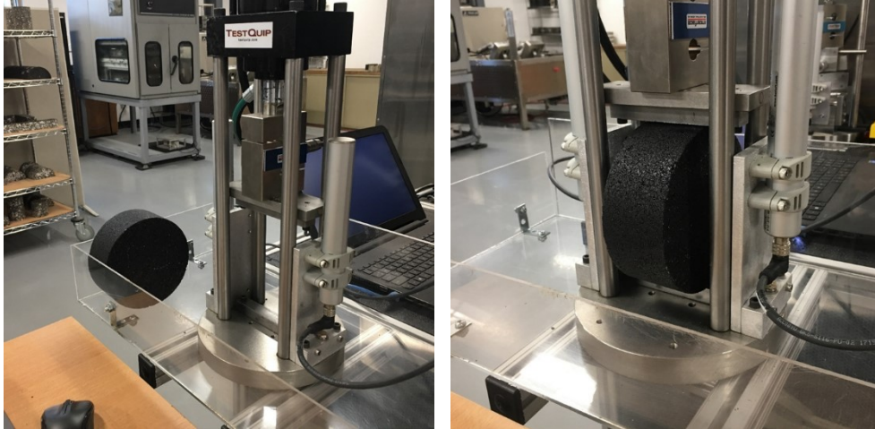
Figure 4. IDEAL-CT Test Device and Specimen Setup
