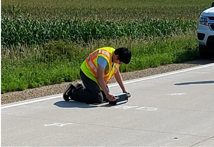
Figure 2.4 Testing of a concrete pavement surface with MIRA
