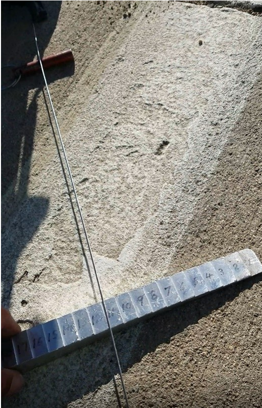
Figure 2.12 Curling measurement performed at slab corner on CSAH 46
