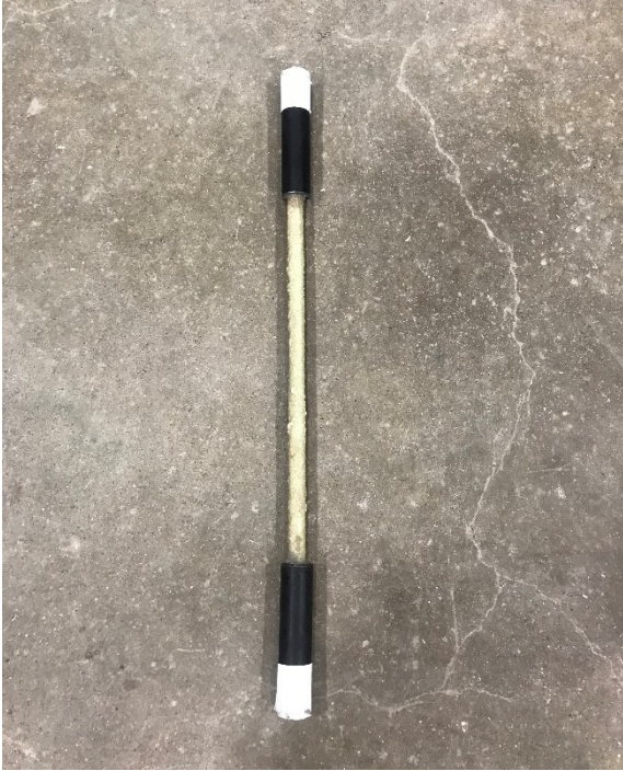
(a) GFRP specimen before testing
