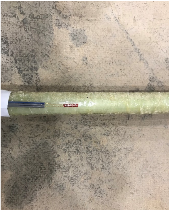
(a) Specimen instrumented with strain gauge
