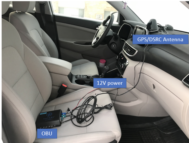
Figure 2.2: OBU installation diagram
