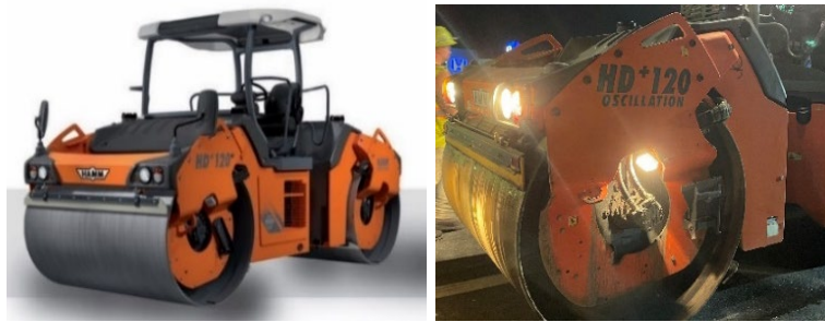
Figure 5. Roller compactor and SmartRock on the drum.
