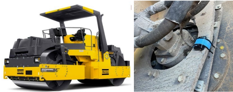
Figure 7. Vibratory roller in Indiana project and the SmartRock on the roller.
