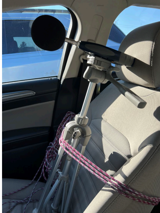
Figure 10. Photo. Equipment setup for internal noise level measurement on US-41.
