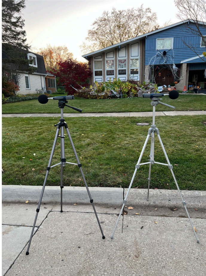
Figure 9. Photo. Equipment setup for external noise level measurement on McCraren Road.
