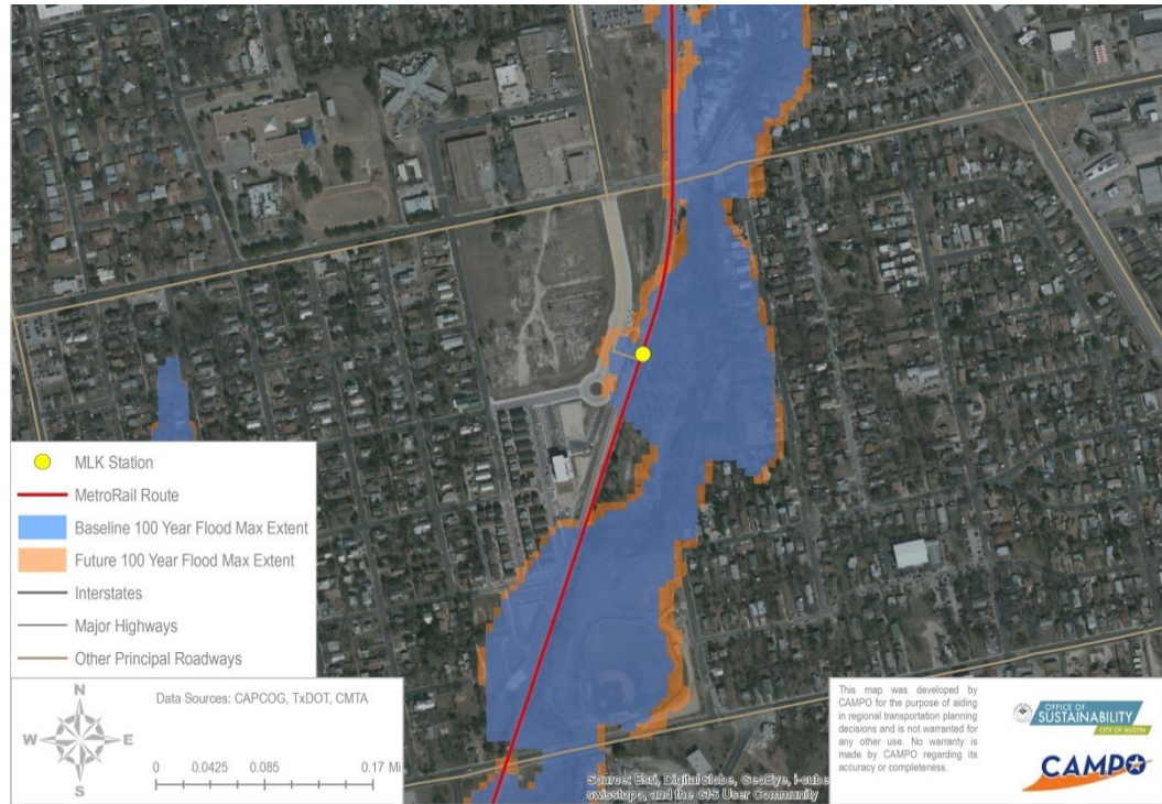
Figure D-1 100 Year Maximum Flood Extents and Cross-section, MetroRail Red Line at MLK Station
