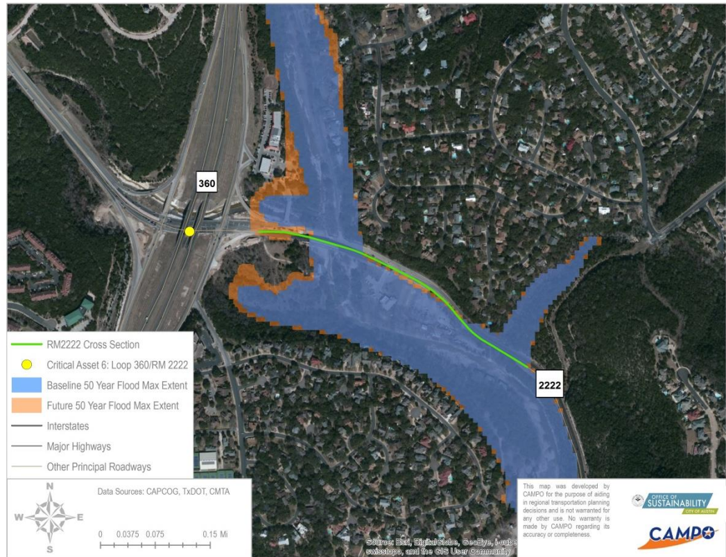
Figure D-12 Projected 50-Year Maximum Flood Extents and Cross-section Location, Loop 360/RM 2222
