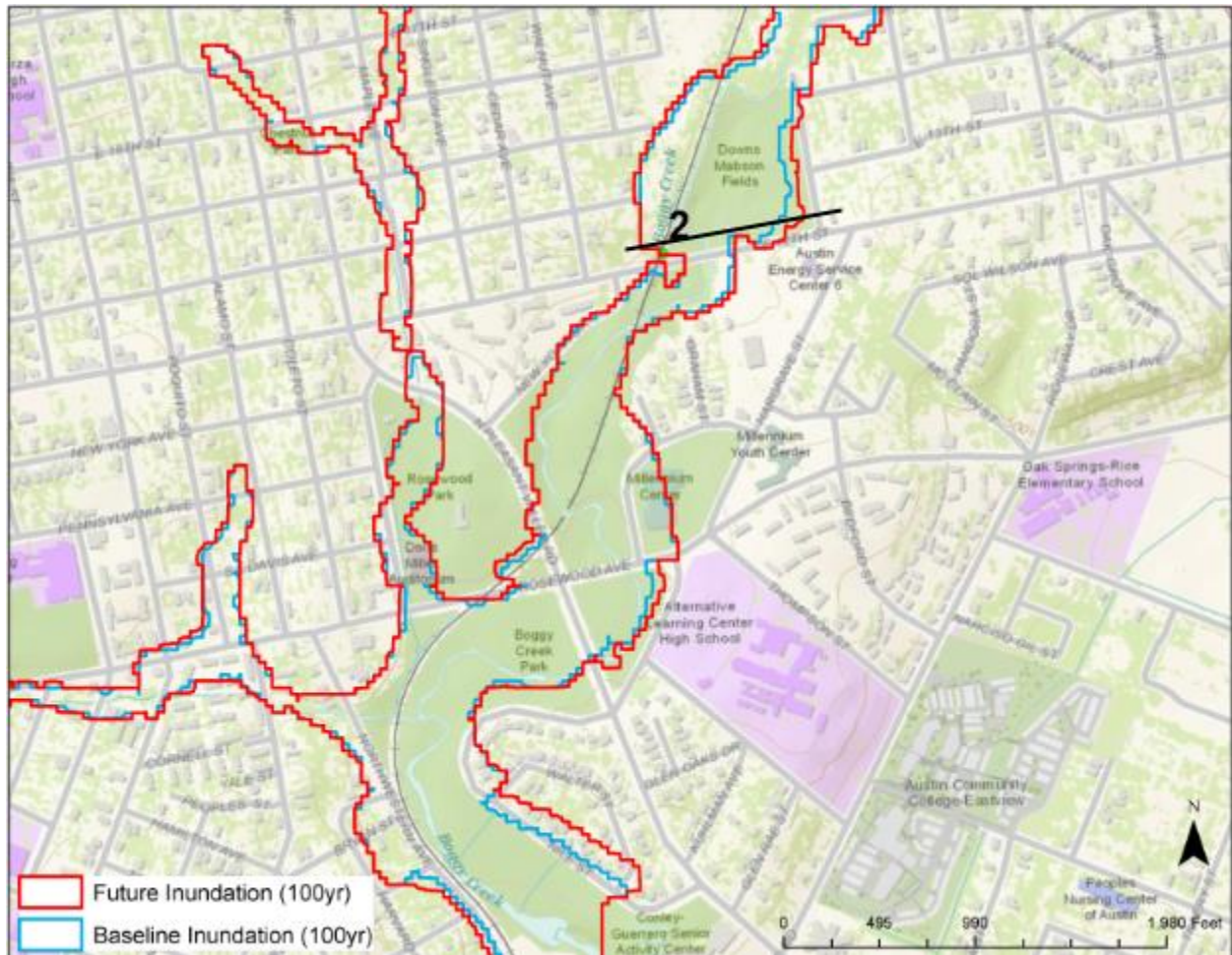
Figure A-2 Inundation extent for baseline (blue) and future (red) 100-yr event at Location 2.
