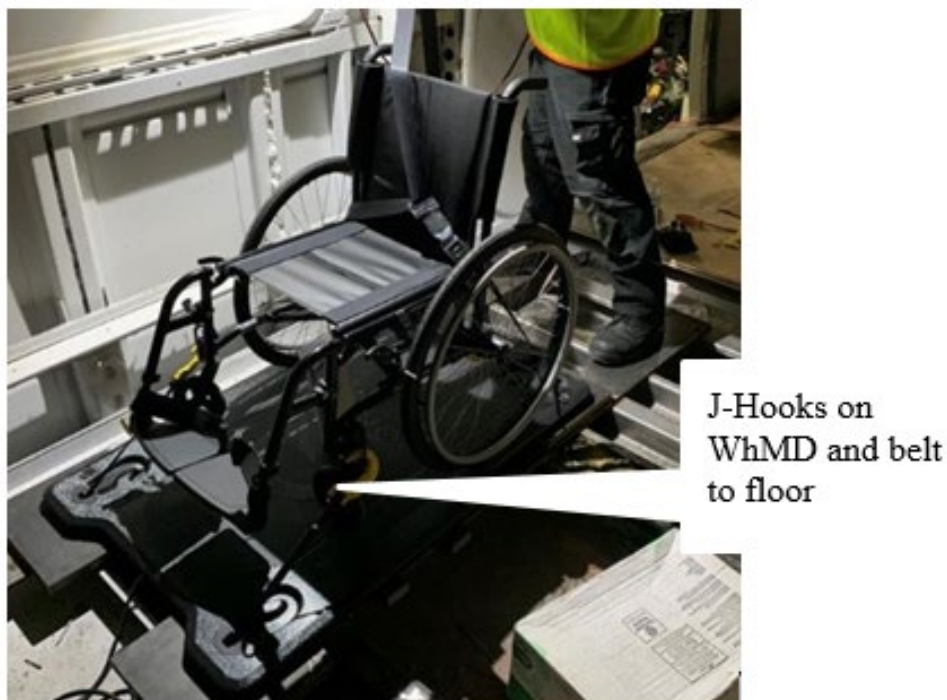
Figure 7. Q'Straint One System (wheelchair shown for demonstration, not the SWC wheelchair that was used in the test)
