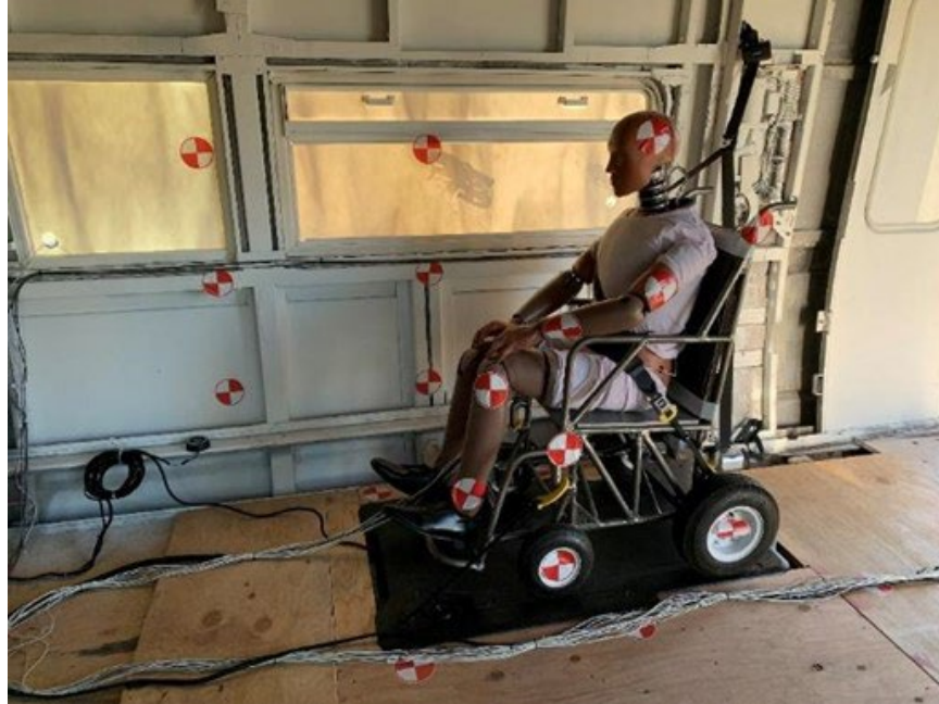
Figure 8. Experiment 2 forward-facing ATD pre-crash final setup
