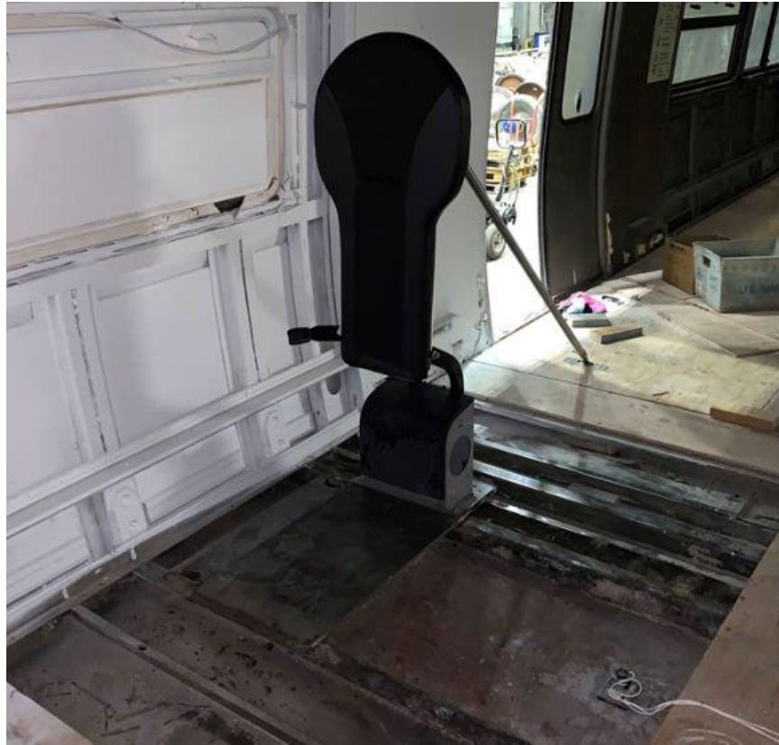
Figure 5. Installation of Quantum backboard restraint device
