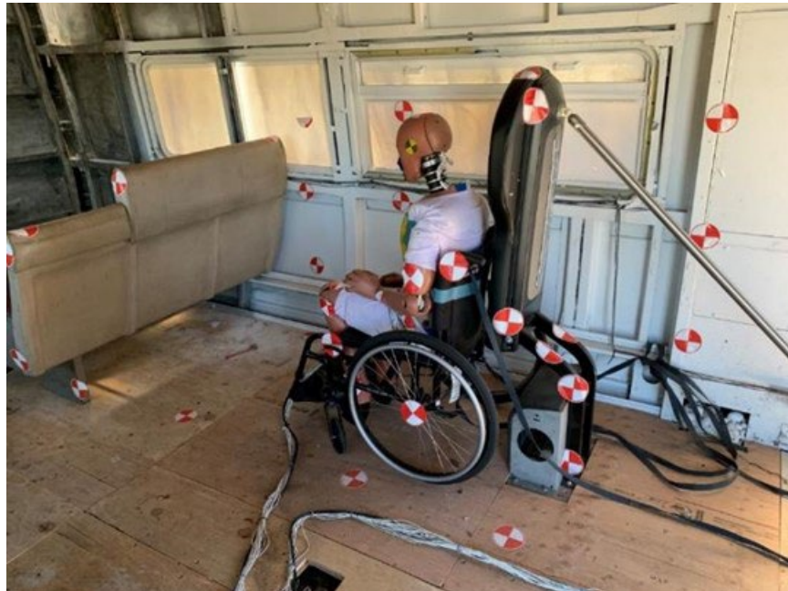
Figure 11. Post impact Unrestrained Quantum backboard
