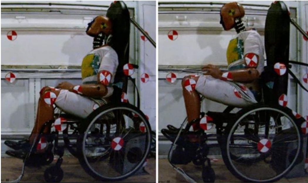
Figure 16. Movement of the ATD rear-facing wheelchair during impact
