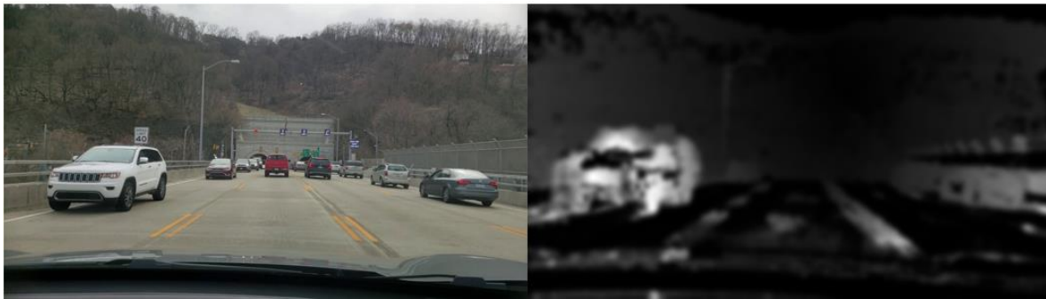
Figure 9 RGB image and corresponding optical flow image.
