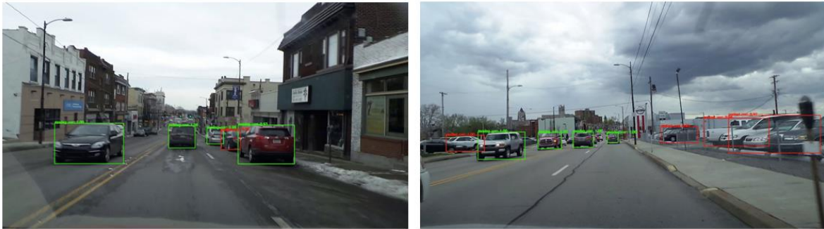
Figure 12 Examples of moving (green) and parked (red) vehicle detection. In the left image are two parked vehicles that are mis-classified as moving and some others in the background that are not classified at all. On the right side one can see many vehicles that are parked off the road.
