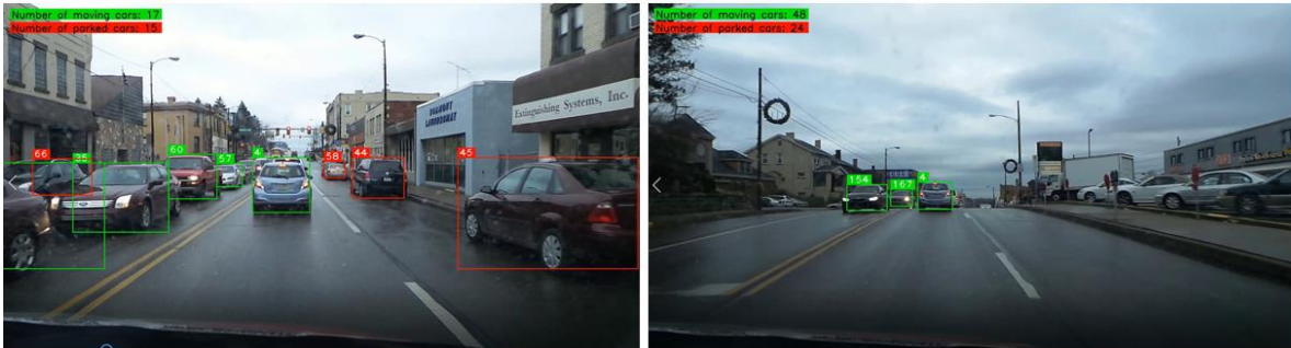
Figure 19 The two images show detection and tracking of moving (green) and parked cars (red). Only cars parked on the road are counted, vehicles in a parking lot on the side are ignored. The boxes around the cars show their ID, the total number of detected and tracked cars are shown in the upper left corner.
