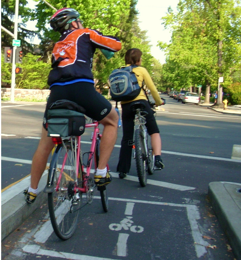
Figure 2. An example of infrastructure used to create a bicycle boulevard (photo credit: Richard Masoner)
