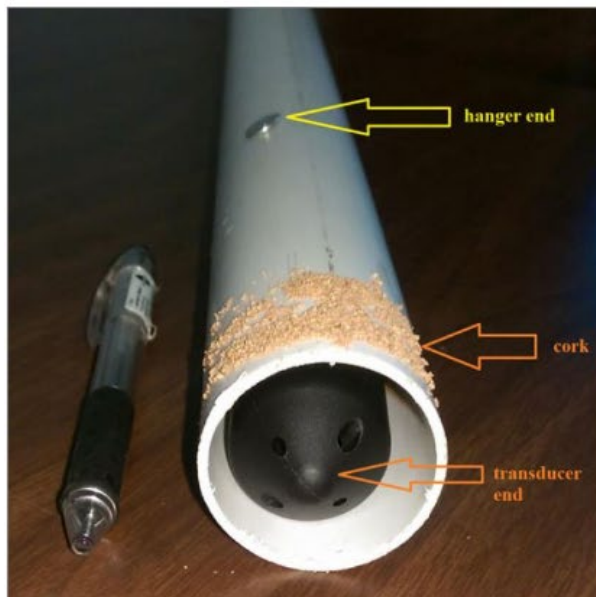
Figure 2. The typical crest-stage gage setup with cork dust and a pressure transducer.
