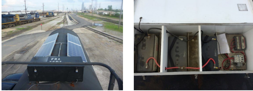
Figure 10. Solar Panel and Battery Box on Top of Instrumented Tank Car
