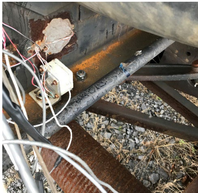
Figure 8. Dual-Axis Accelerometer Mounted on the Stub Sill at Each End of the Car
