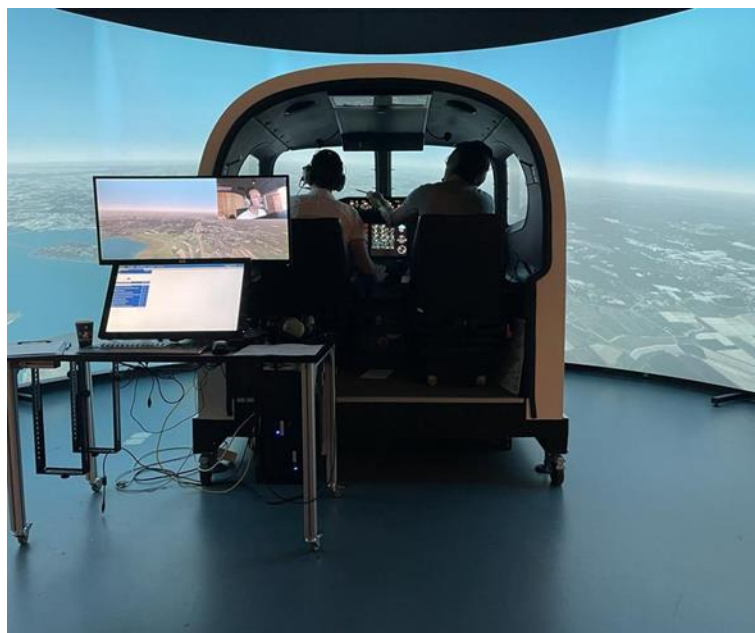
Figure 1. Fixed-base simulator with participant in the left seat, and instructor in the right seat
