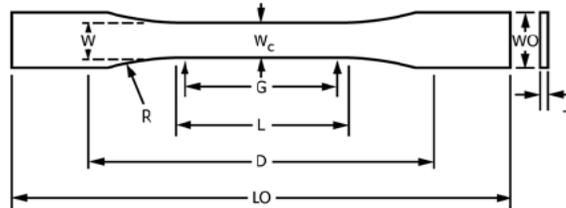
Figure 6. Plastic tension specimen geometry
