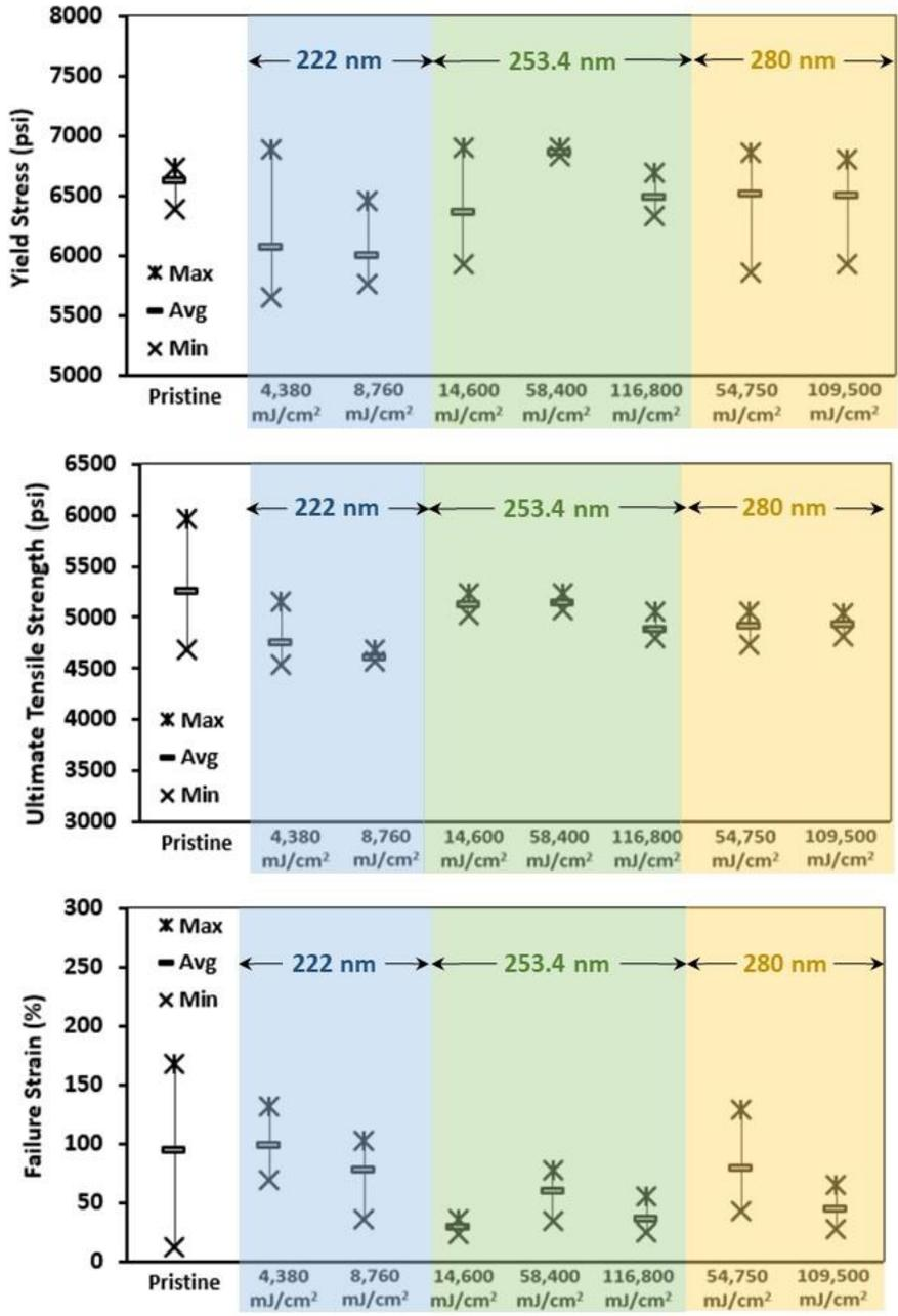
Figure 15. Yield stress, ultimate tensile strength, and failure strain – Boltaron 9815N
