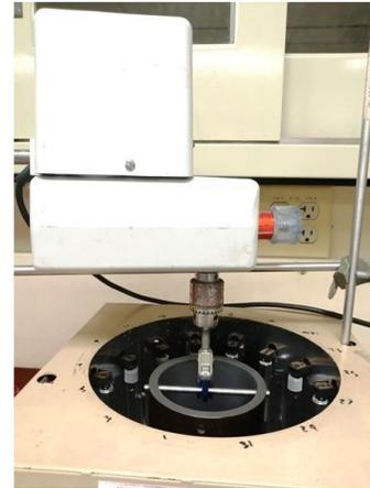
Figure 3. UV-C test setup with 253.4 nm lamps – Rayonet Reactor
