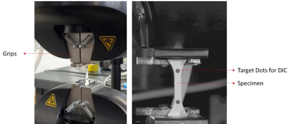
Figure 7. Tensile test setup - Plastics
