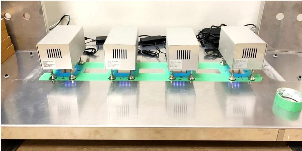
Figure 2. UV-C test setup with Ushio Care222 nm lamps
