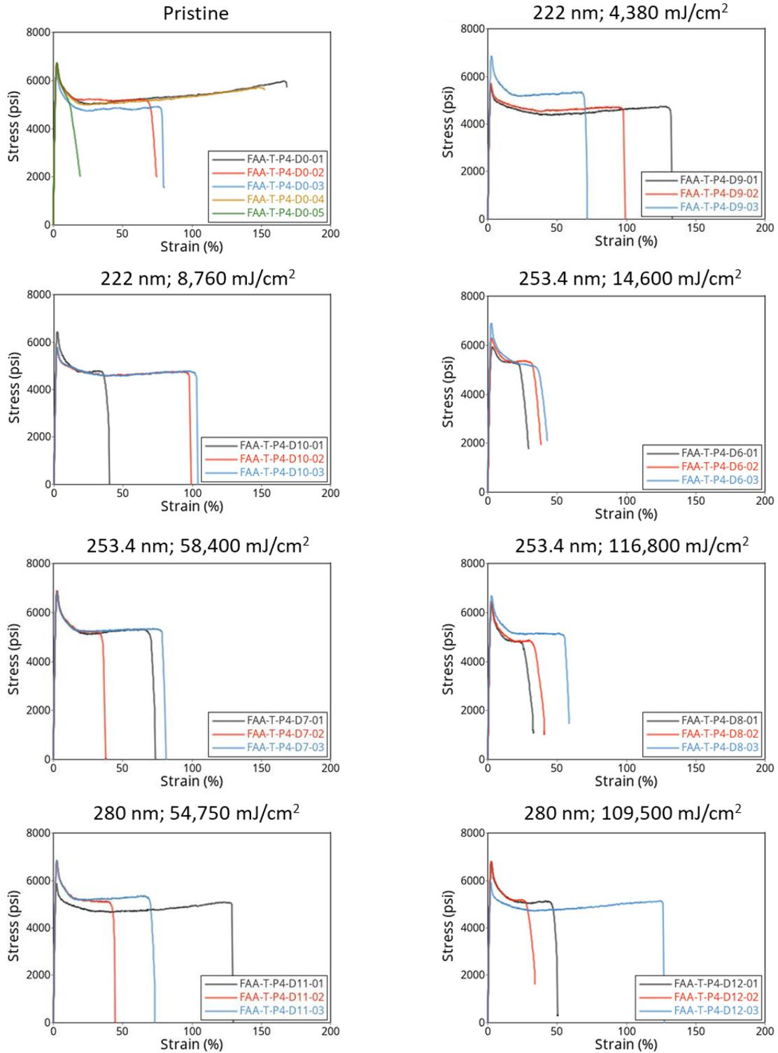
Figure 14. Longitudinal stress-strain response – Boltaron 9815N
