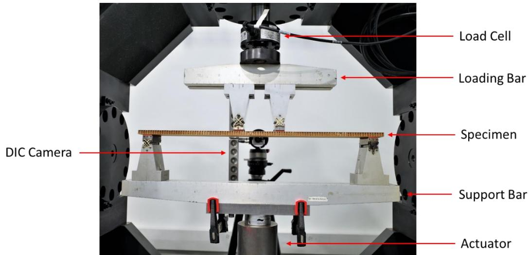
Figure 21. Long-beam flexure test setup
