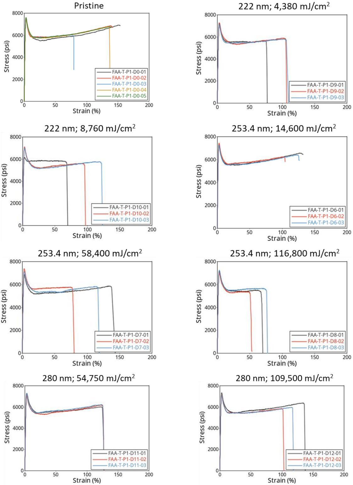
Figure 8. Longitudinal stress-strain response – Kydex 6565
