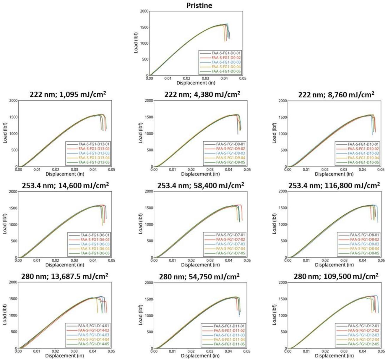
Figure 26. Load-displacement response – Fiberglass G-10/FR4
