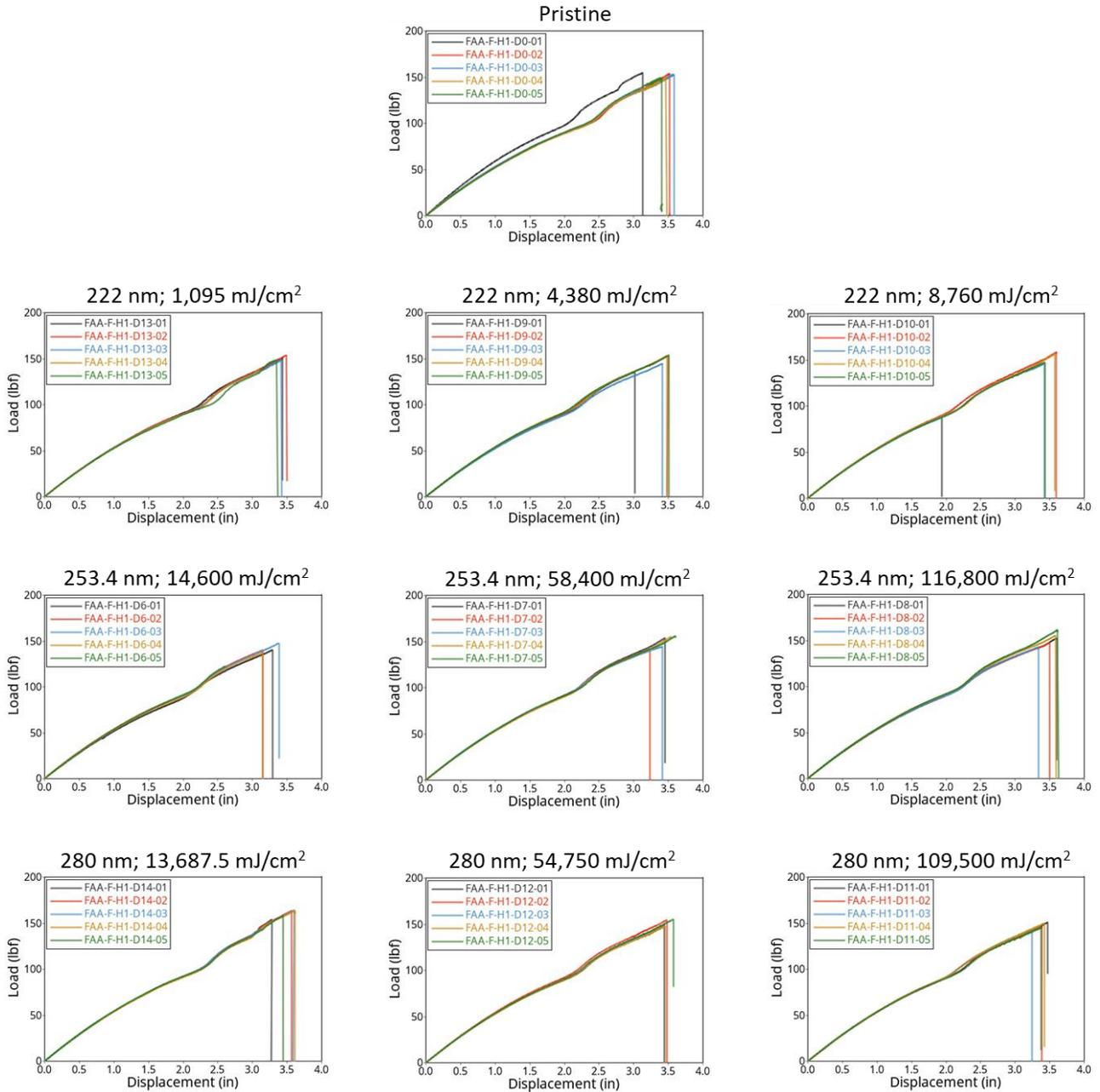
Figure 22. Load-displacement response – Honeycomb type A
