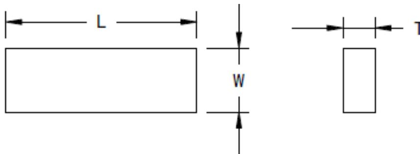
Figure 24. Short-beam shear specimen geometry
