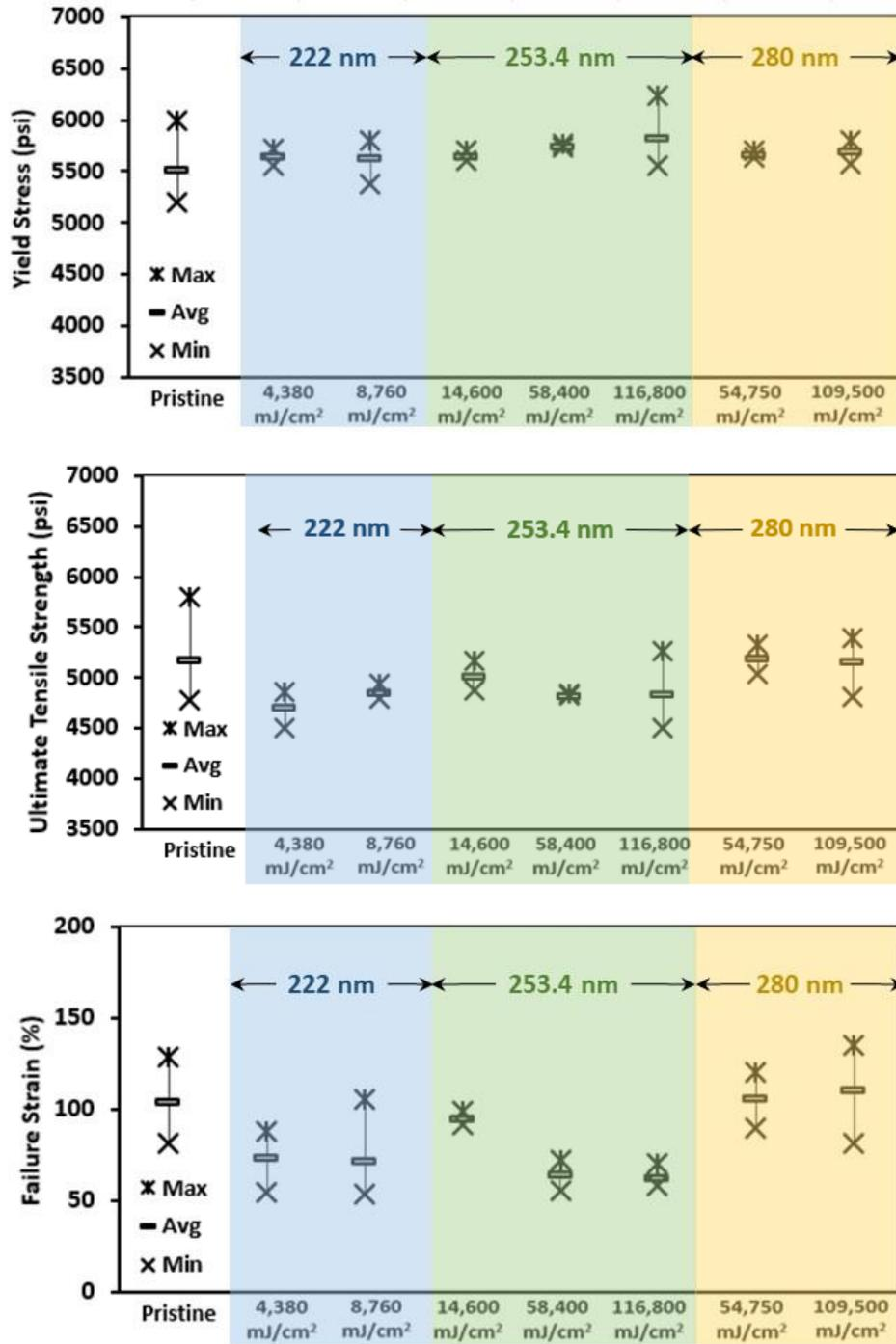
Figure 11. Yield stress, ultimate tensile strength, and failure strain – Boltaron 9815E
