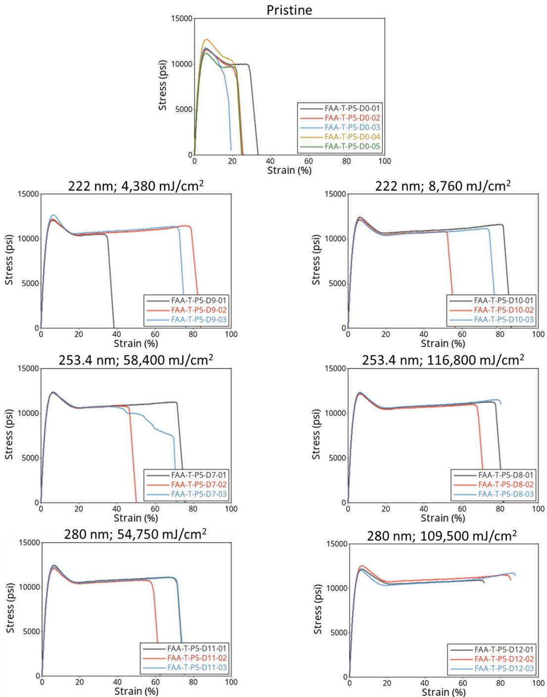
Figure 16. Longitudinal stress-strain response – ULTEM™ 9075
