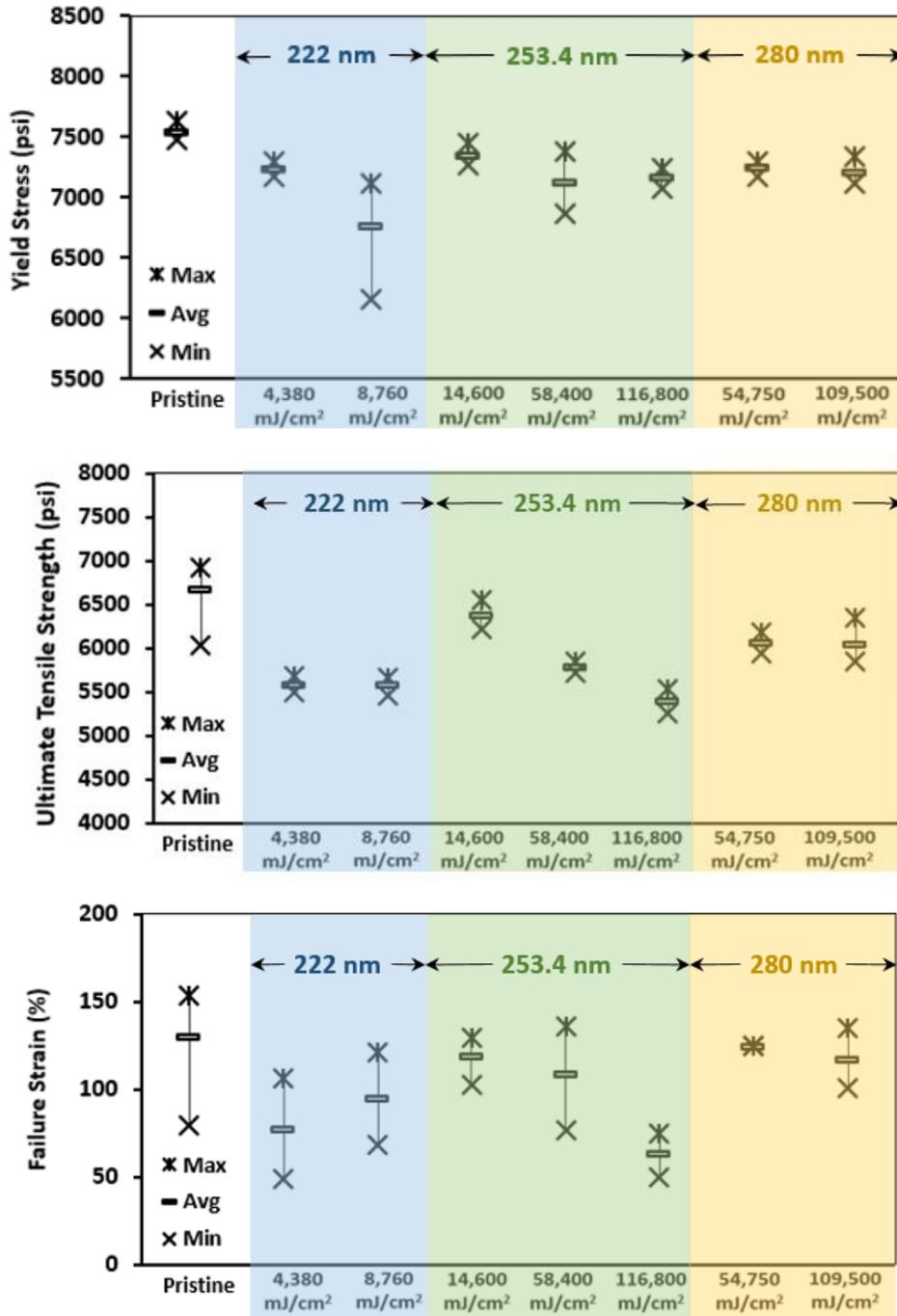
Figure 9. Yield stress, ultimate tensile strength, and failure strain – Kydex 6565
