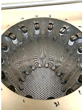
253.4 lamps inside the Rayonet reactor barrel
