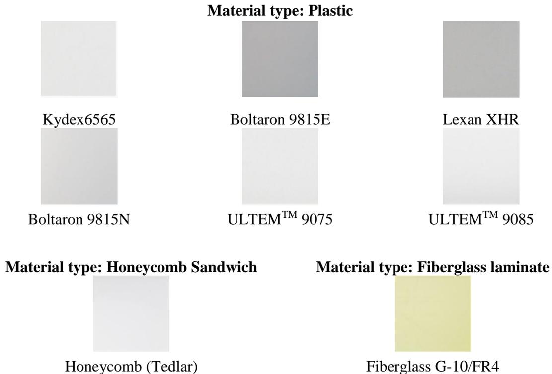
Figure 1. Materials evaluated for accelerated aging tests with UV-C exposure
