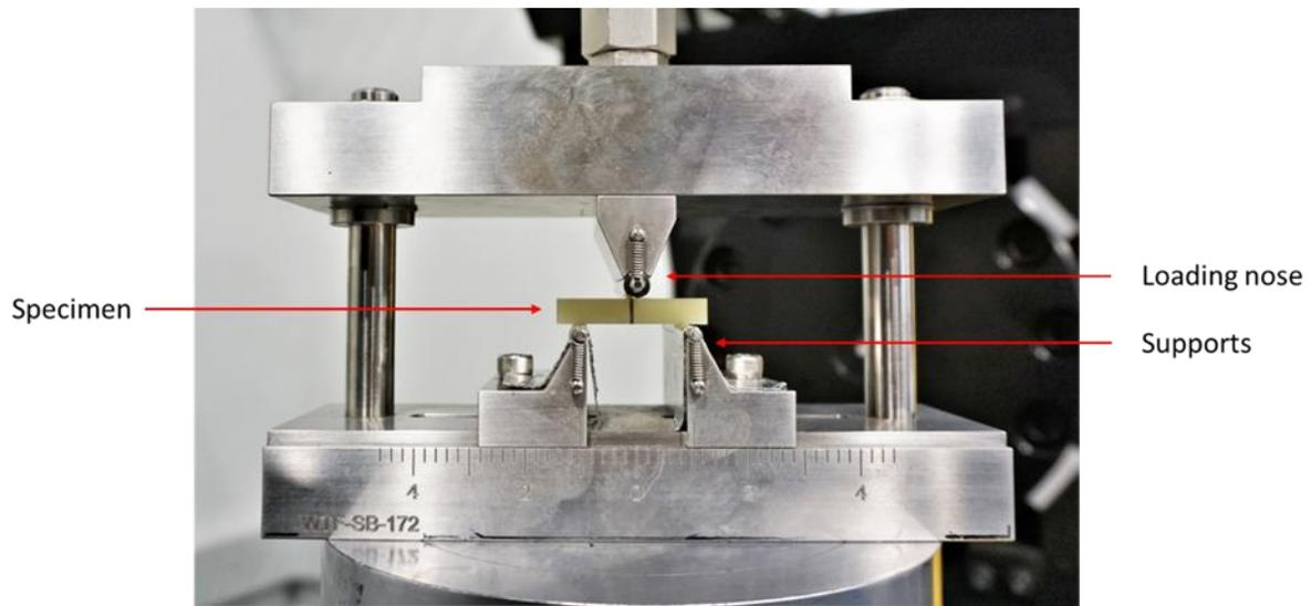
Figure 25. Short-beam shear test setup
