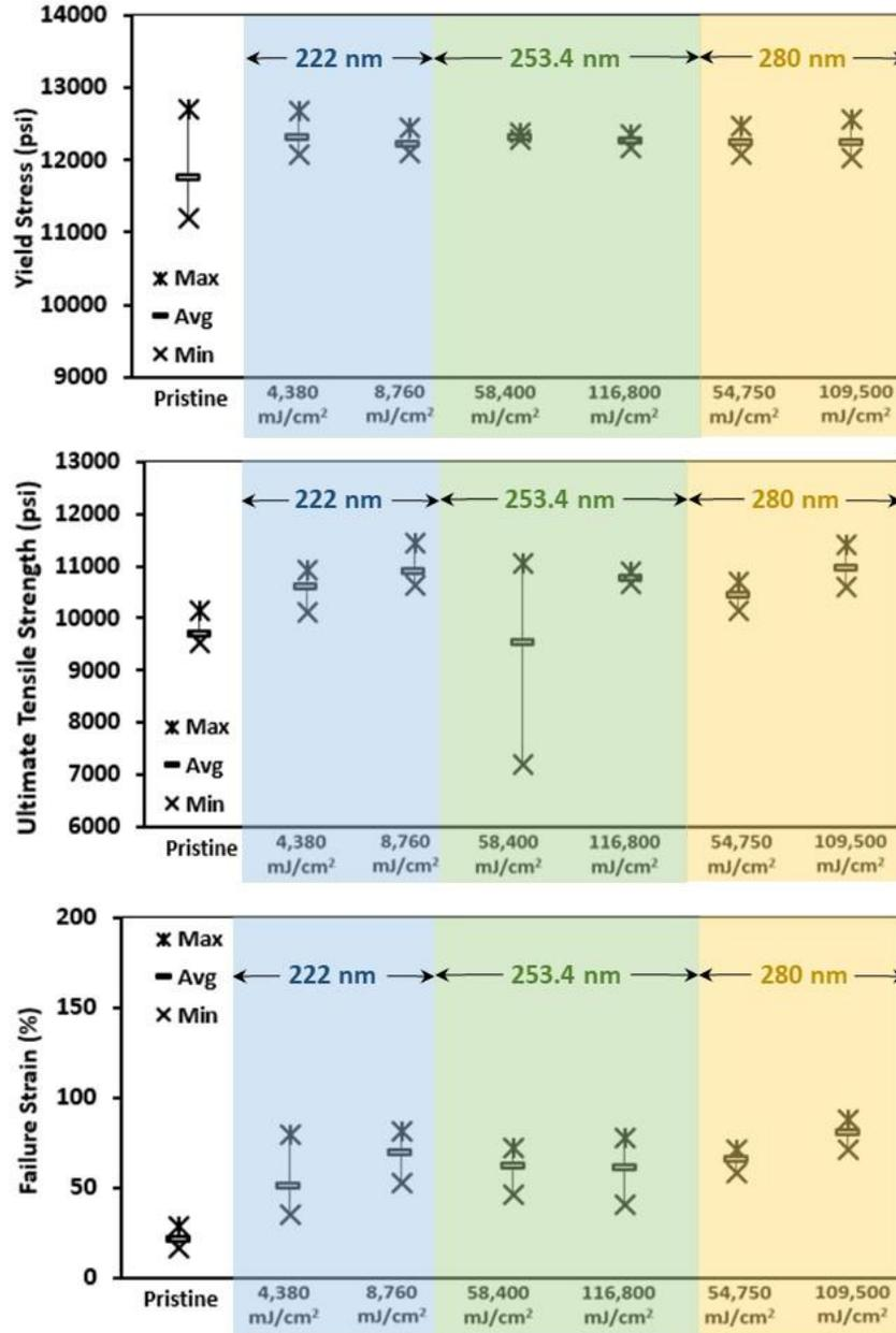
Figure 17. Yield stress, ultimate tensile strength, and failure strain – ULTEM™ 9075
