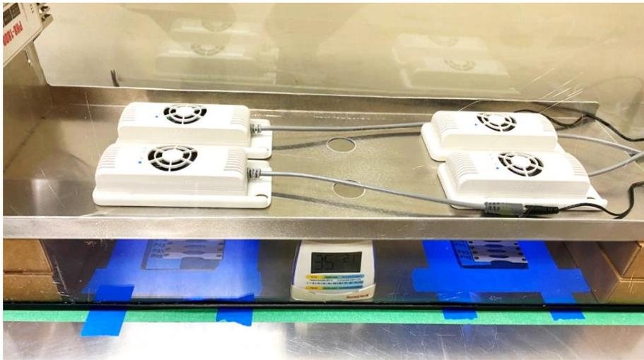
Figure 5. UV-C test setup with Aquisense 24G UVinaire 280 nm LED lamp modules
