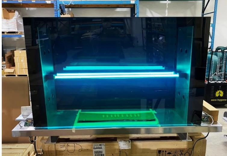
Figure 4. UV-C test setup with 253.4 nm lamps – LightTech
