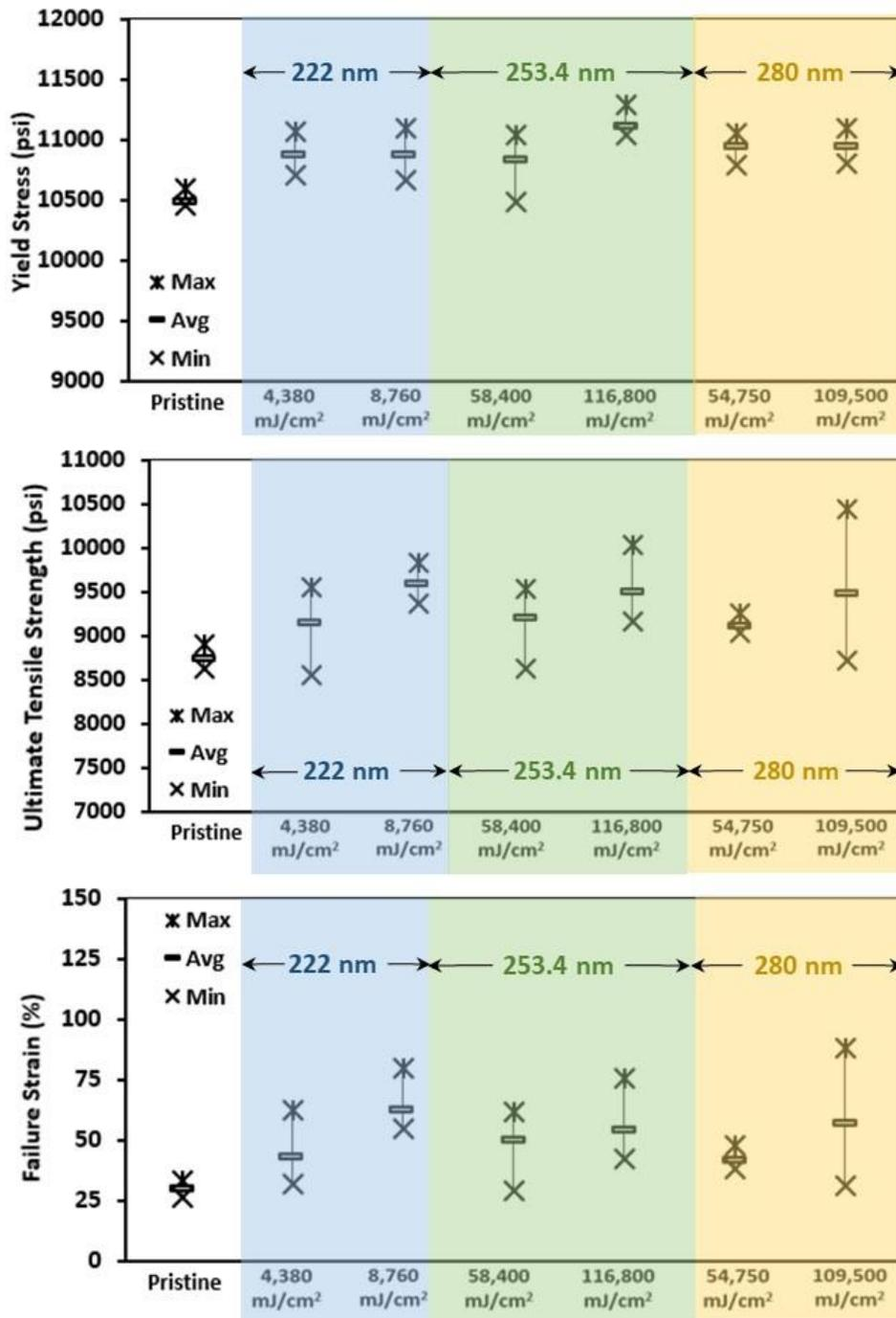
Figure 19. Yield stress, ultimate tensile strength, and failure strain – ULTEM™ 9085
