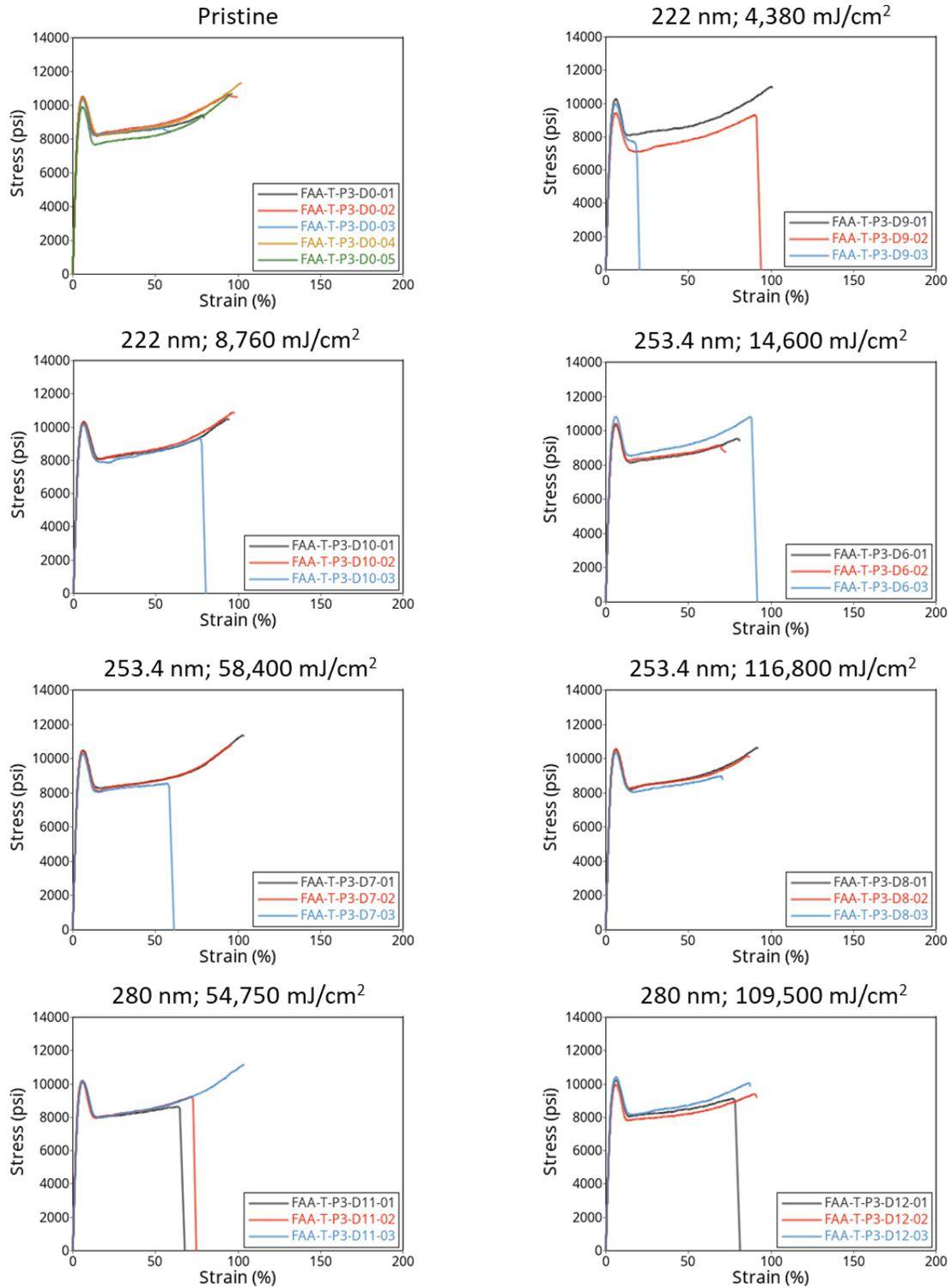
Figure 12. Longitudinal stress-strain response – Lexan XHR
