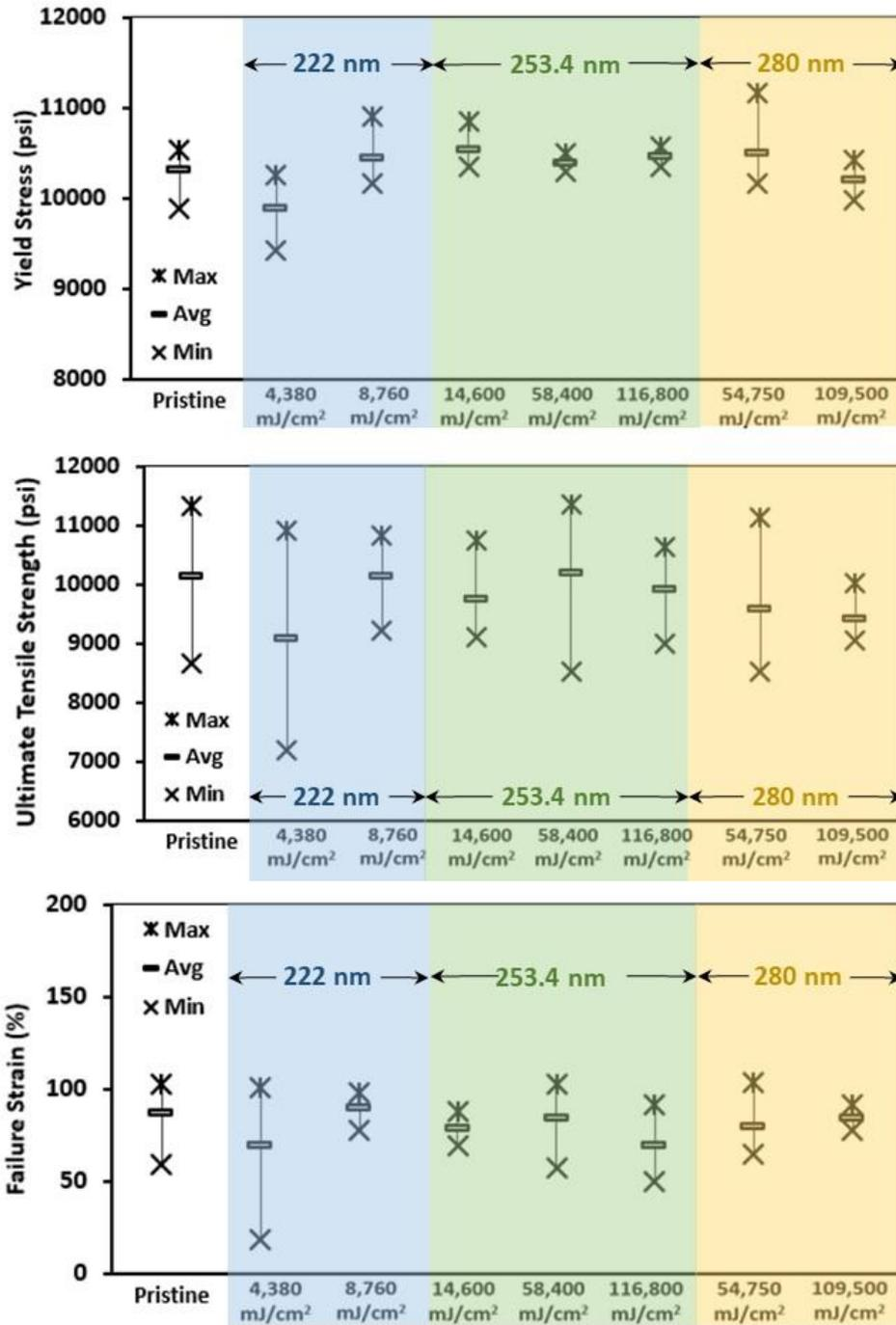
Figure 13. Yield stress, ultimate tensile strength, and failure strain – Lexan XHR
