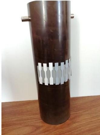
Test specimens taped to the pipe and suspended into the reactor barrel
