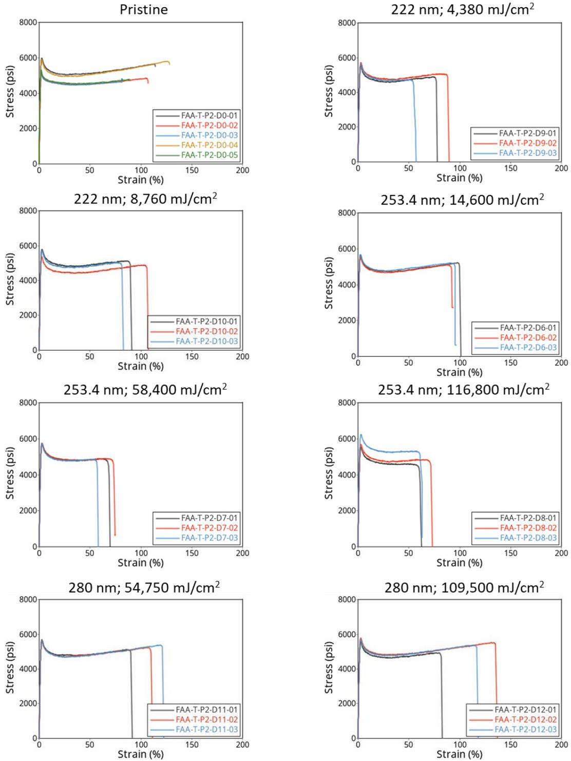
Figure 10. Longitudinal stress-strain response – Boltaron 9815E
