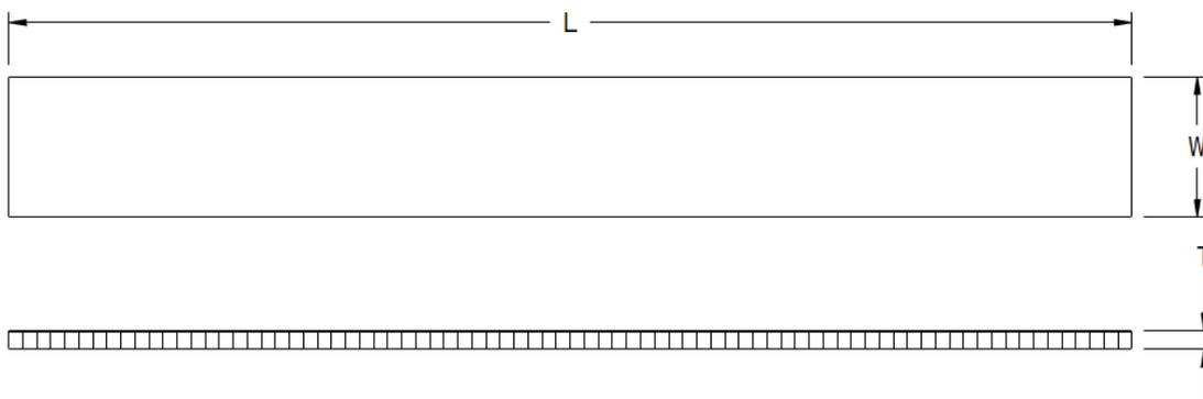
Figure 20. Long-beam flexure specimen geometry
