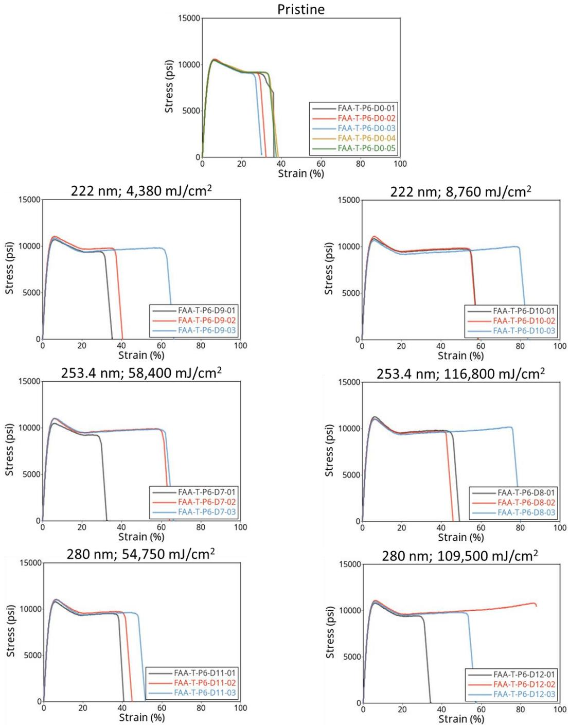
Figure 18. Longitudinal stress-strain response – ULTEM™ 9085
