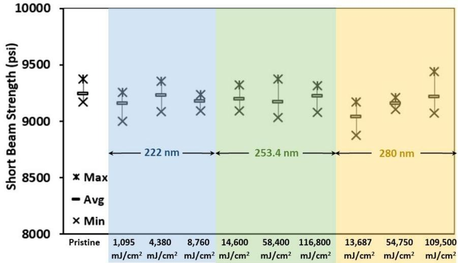
Figure 27. Short-beam strength comparison – Fiberglass G-10/FR4
