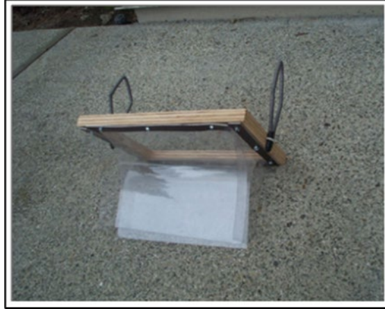
Figure 6. Photo of one-way door used to exclude bats from expansion joints and hinges (Photo used with permission from H.T. Harvey & Associates and HDR 2021).
