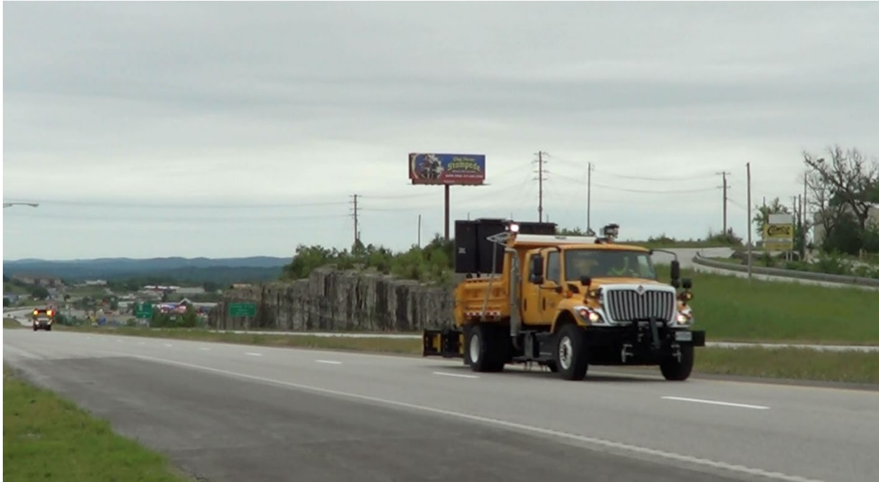
Figure 4-3. Leader-Follower TMA system traveling on US 65 near Branson, Missouri
