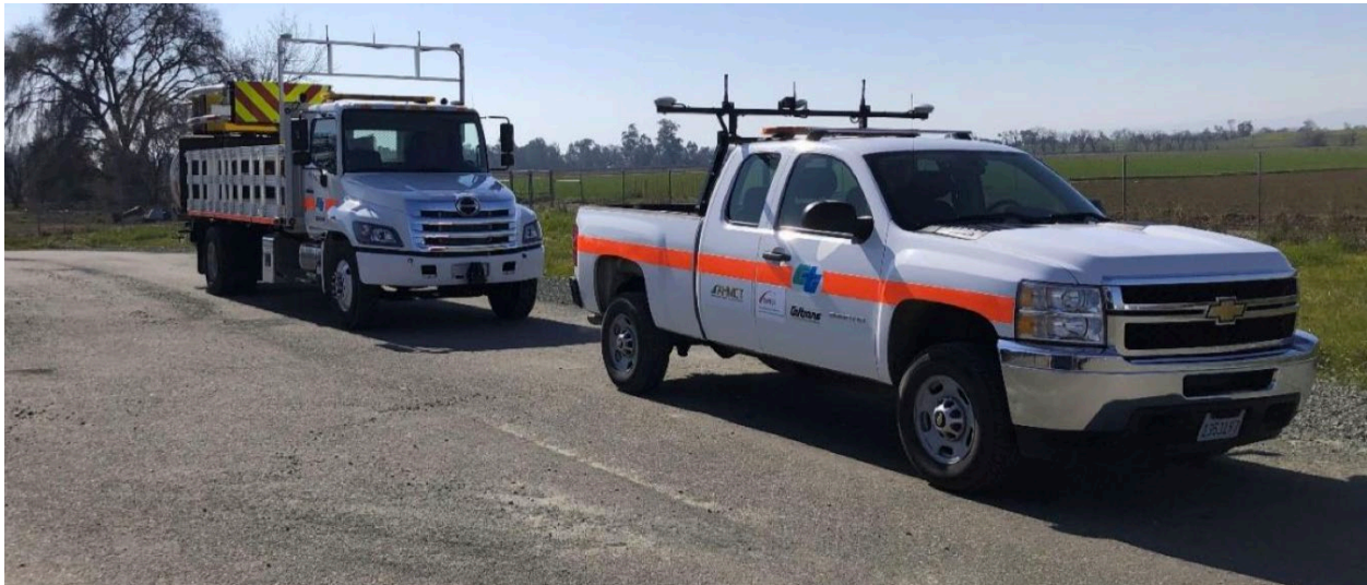
Figure 2-2. Leader-Follower TMA configuration for Caltrans study
