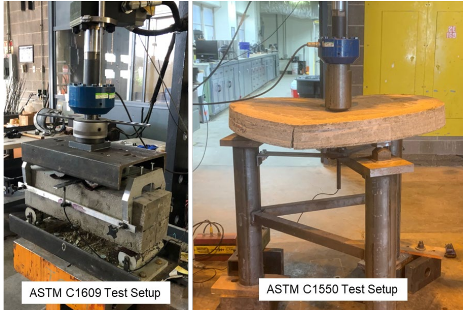
Figure 22. A schematic of ASTM test setups to evaluate flexural toughness of FRC mixtures
