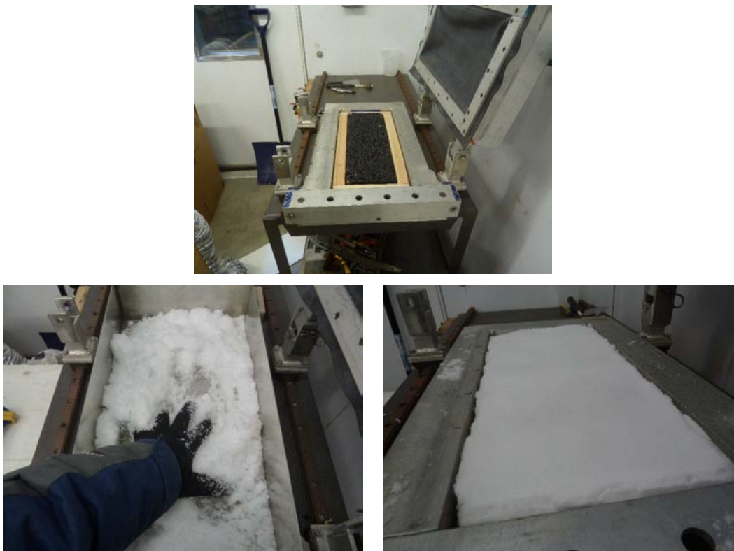
Figure 2.2 Snow production, sieving and compaction
