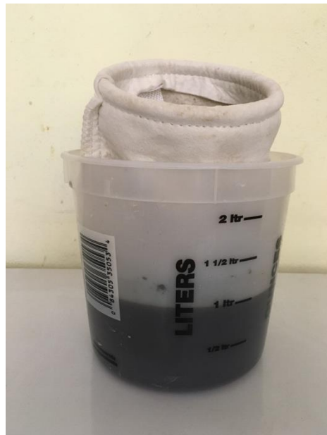
Figure 2.3 Fly ash in filter bag soaking in GO suspension
