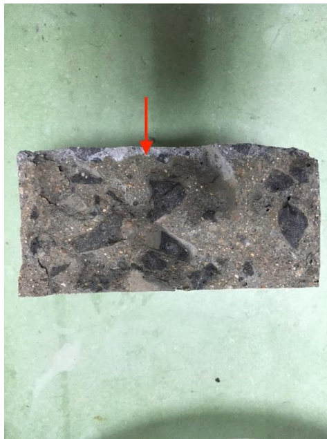
Figure 3.9 Precipitated chlorides after treatment with silver nitrate (arrow indicates precipitated chlorides reaction front)
