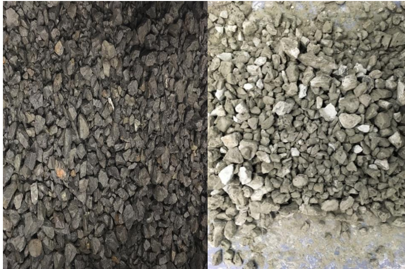
Figure 3.2 Coarse aggregate before and after (left to right) surface treatment using cement slurry
