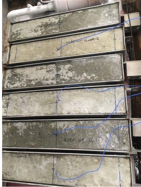
Figure 3.3 Thermocouples embedded concrete samples in the F-T chamber
