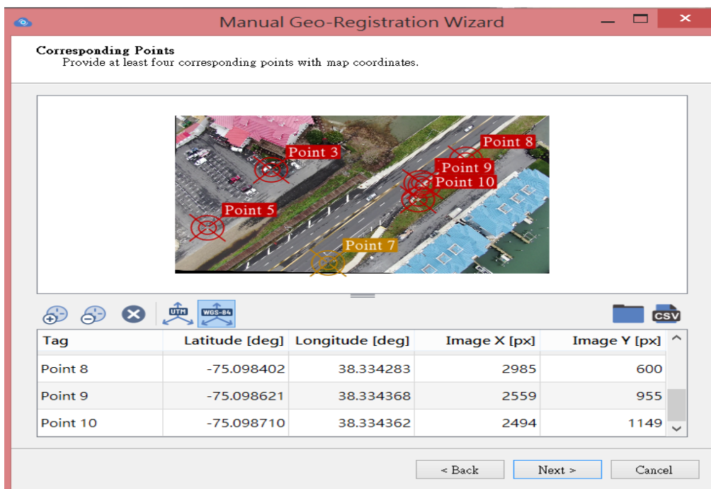
Figure 2-2: Example of geo-registration to match the target roadway segment in the drone's video with its real-world coordinates
