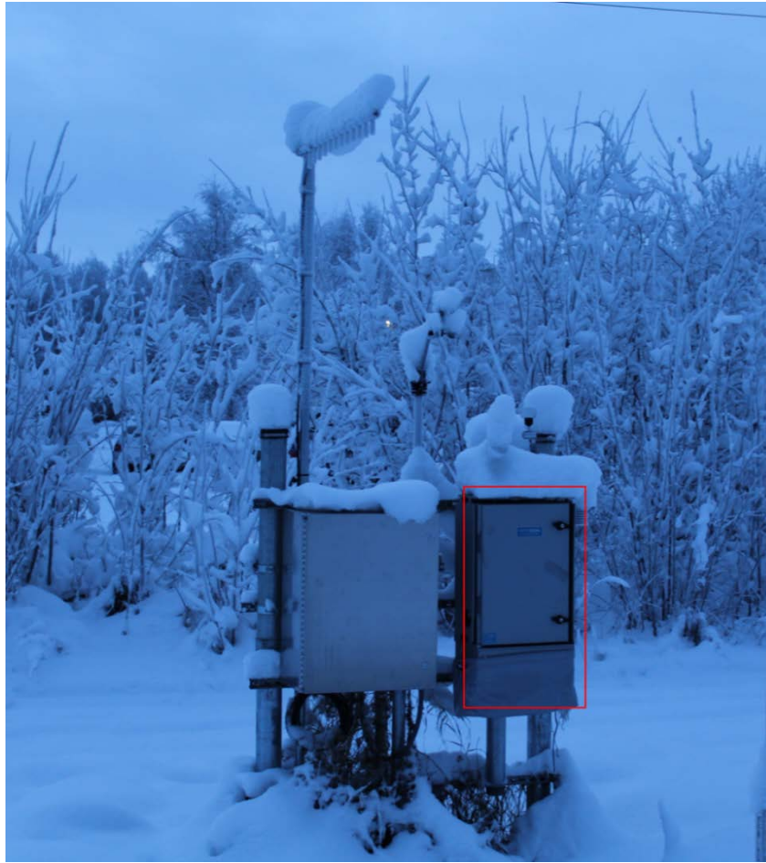
Figure 3.3 RWIS site equipped with AQM60 air quality monitor (rectangular box outlined in red) with other road weather monitoring devices
