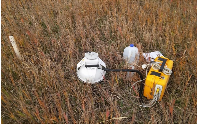
Figure 16. LI-COR® Biosciences LI-8100A gas analyzer used to measure carbon loss from soils on individual experimental plots.
