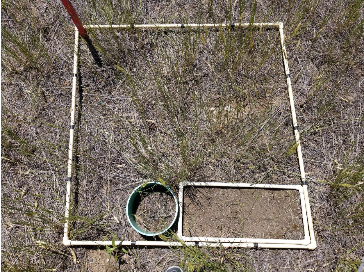
Figure 15. A sample of vegetation and litter was collected from a 20 cm × 50 cm quadrat (bottom right) placed randomly within the 1 m 2 plot for lab tests to determine the amount of aboveground carbon of plots. A 10 cm ring of 20 cm diameter round pipe was installed permanently in each 1 m 2 plot to serve as a “collar” for soil respirometry measurements (bottom center).
