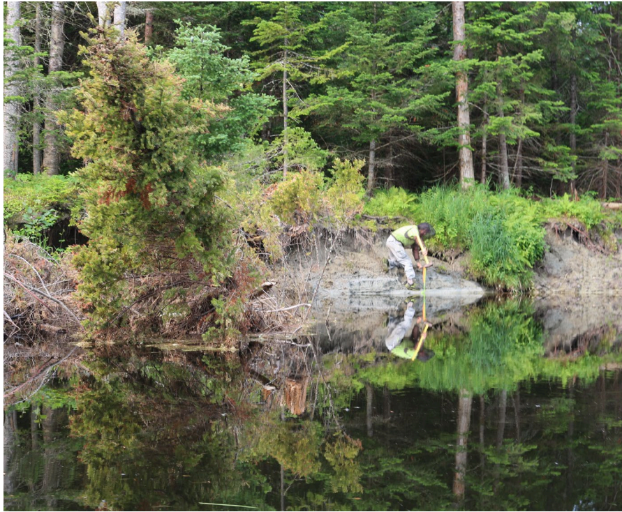
Figure 15. Installation of erosion pin EP R3 at Campground site.
