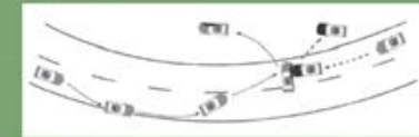
This is a typical diagram for a crash caused by tire scrubbing. The vehicle at left scrubbed the edge of the pavement, and when it returned, the driver overcorrected, lost control, crossed into the adjacent lane, and struck an oncoming vehicle. (Graphic source: AAA Foundation for Highway Safety)
