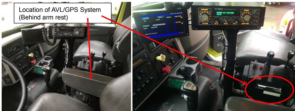
Figure 14. WSDOT Snow Plow Equipment and Location of LT6 AVL/GPS System
