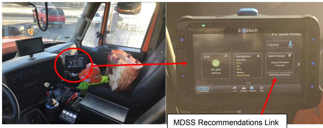
Figure 36. CDOT Snow Plow and Zonar System Tablet Installation Location / Screen
