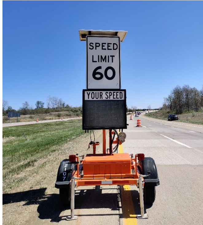
Figure 9. Speed feedback trailer at a work zone lane closure
