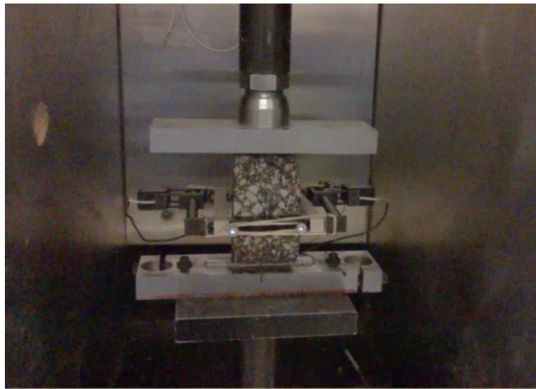
Figure B.1. Indirect Tensile Strength Test Setup
