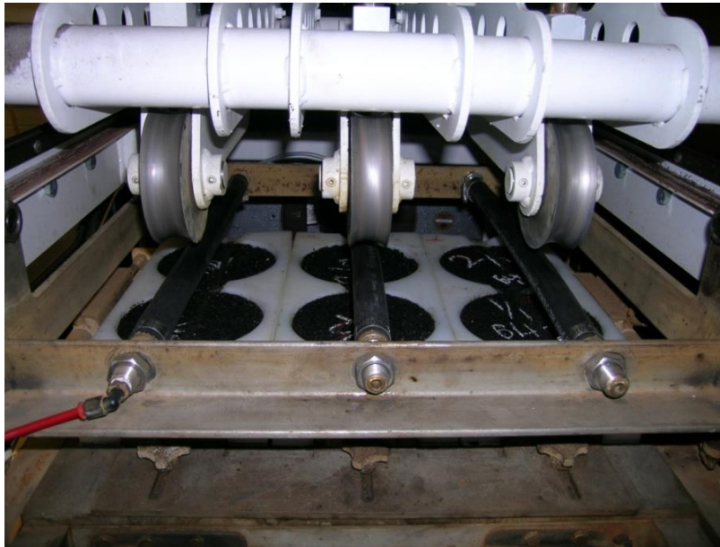
Figure B.4. Repeated Wheel Loading in the APA Device
