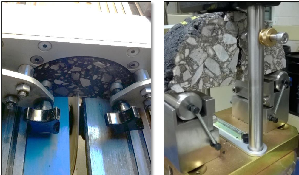
Figure A.5 Illinois SCB Sample Preparation and Testing Equipment
