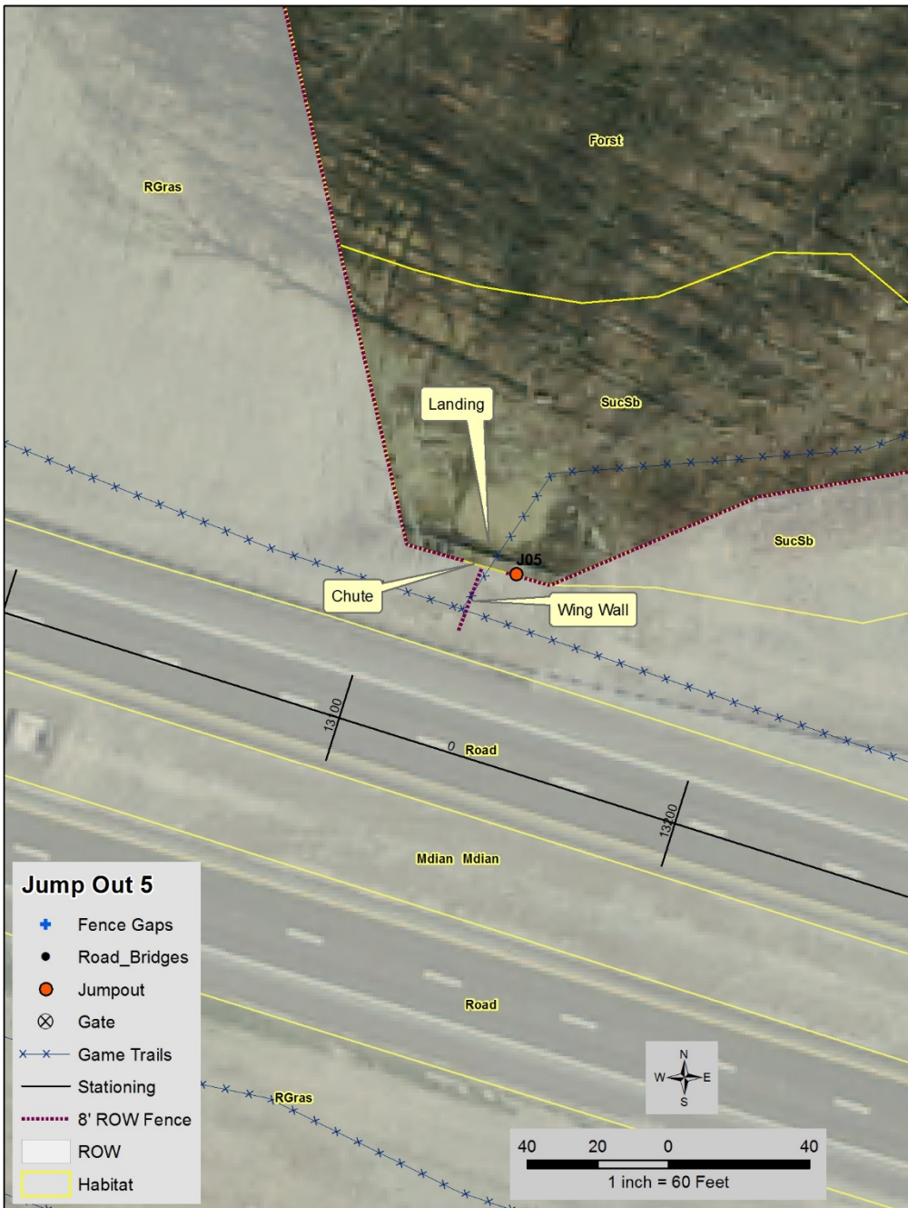
Figure 2-21. Schematic of Jump Out 5 showing wing walls, escape chute, and landing pad. Habitat mapping codes are in Table 2-1.
