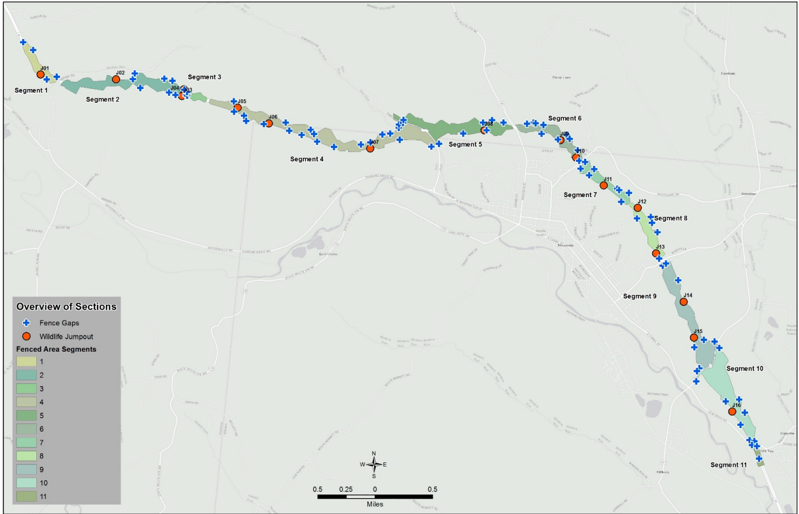
Figure 2-2. Map of the area within the U.S. 33 Nelsonville Bypass right-of-way (ROW). Road segments 1-11 are labeled and color coded. The map also depicts the locations of the one-way jump out mitigation structures (red dots) and fence gaps (blue plus signs).
