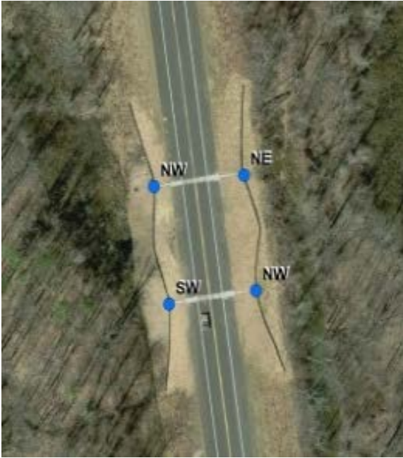
Figure 5-1. Aerial view of the barrier-ecopassage system in place along State Route 78, Athens County, Ohio.
