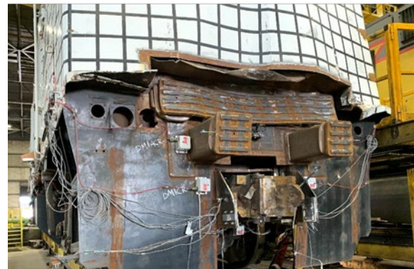
Figure 4 Post-test FEA results (top) vs post-test photo of the CEM locomotive
