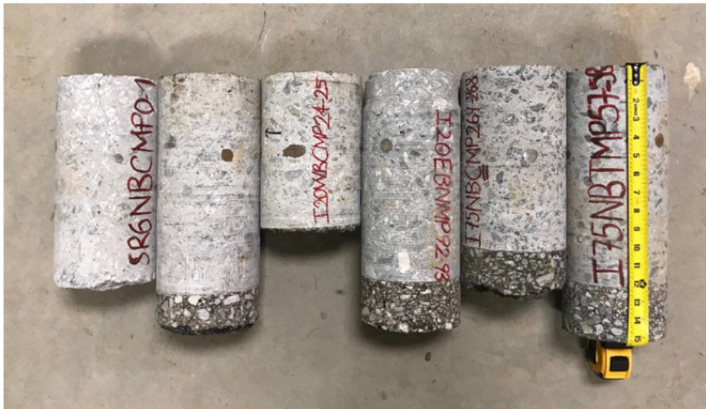
Figure 26 – Core Specimens taken from Site Investigations.
