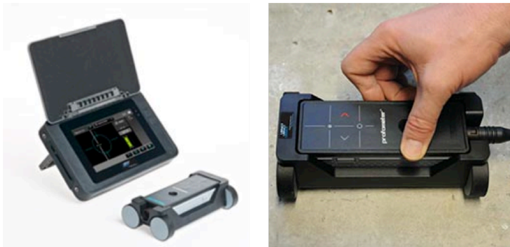
Figure 16 – The Covermeter - Profometer 600 (Impact Test Equipment 2017)
