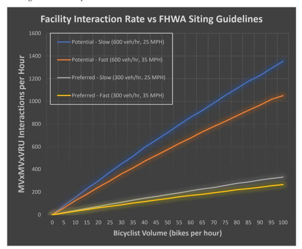
Figure 11. Facility MV×MV×VRU Interaction Rates under FHWA Guidelines
