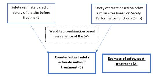
Figure 12. EB-Based Before-and-After Evaluation Framework
